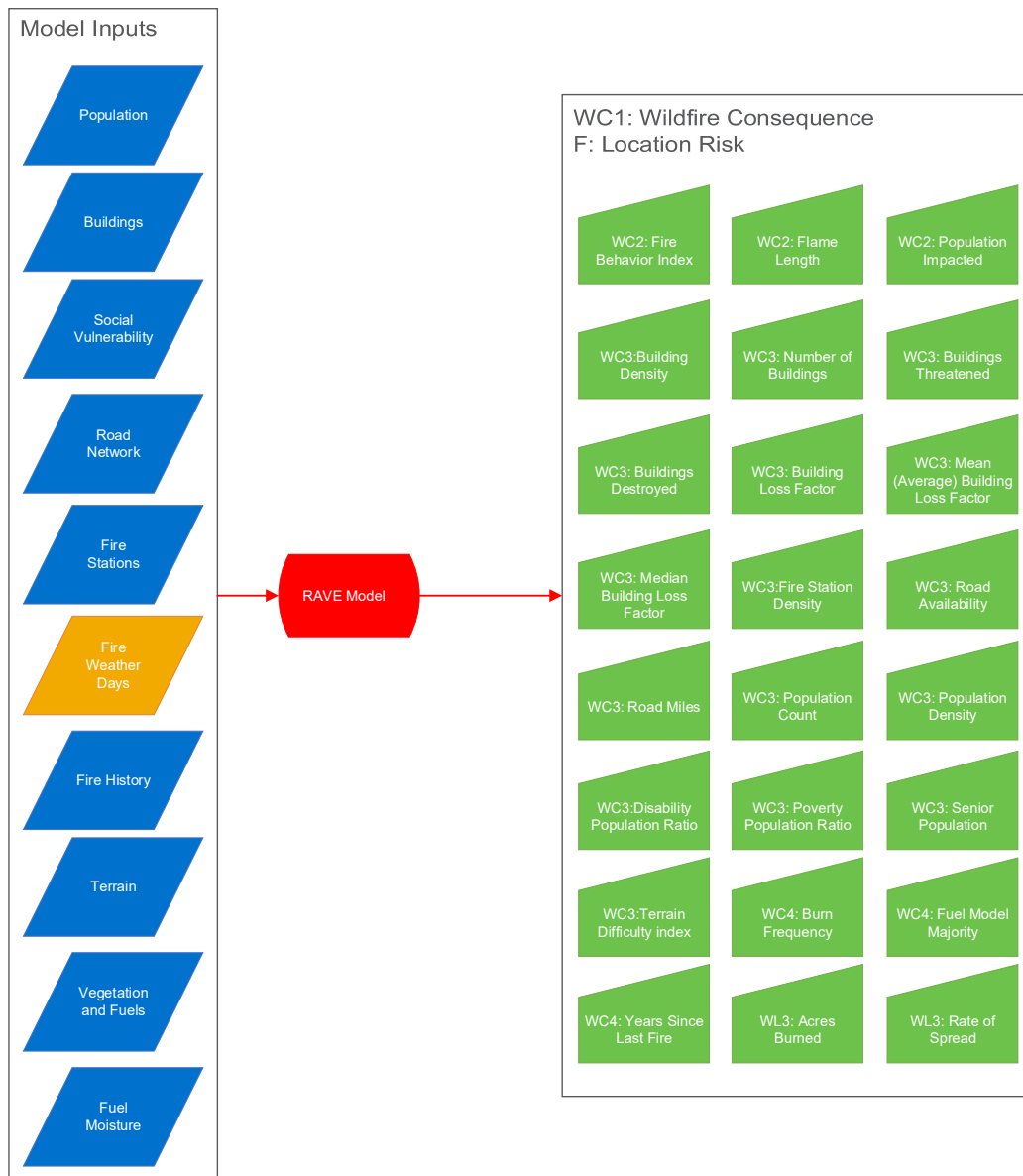
Figure 0-2: Risk Associated with Value Exposure (RAVE) Bowtie Model
