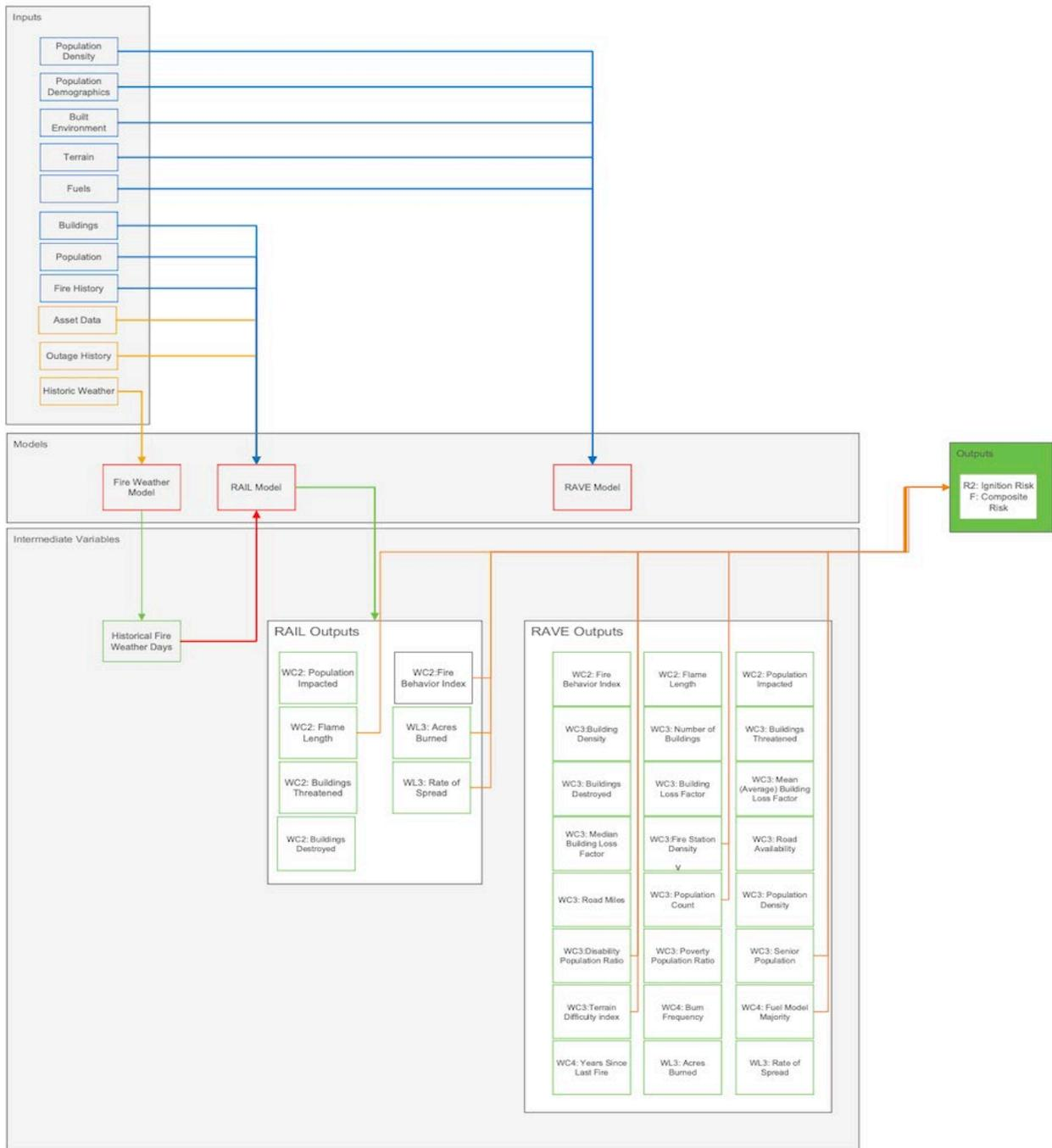
Figure 5-2: FireSight Calculation Schematic
