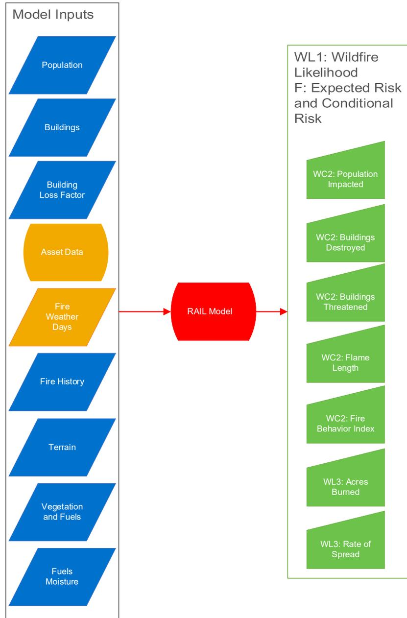
Figure B-1: Risk Associated with Ignition Locations (RAIL) Bowtie Model
