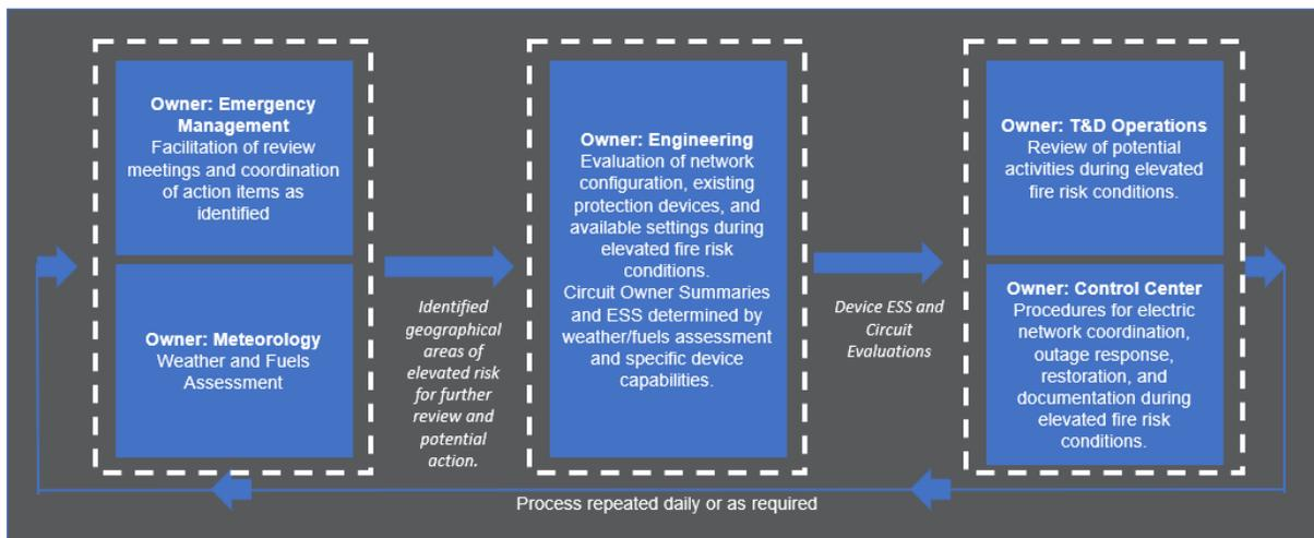
Figure PAC 8-2: Operational Process for ESS Implementation
