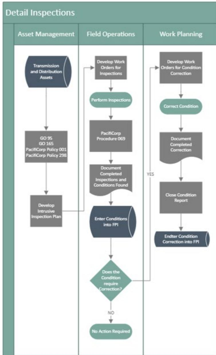
Figure 8-2: Detailed Inspections of Transmission and Distribution Electric Lines and Equipment Workflow
