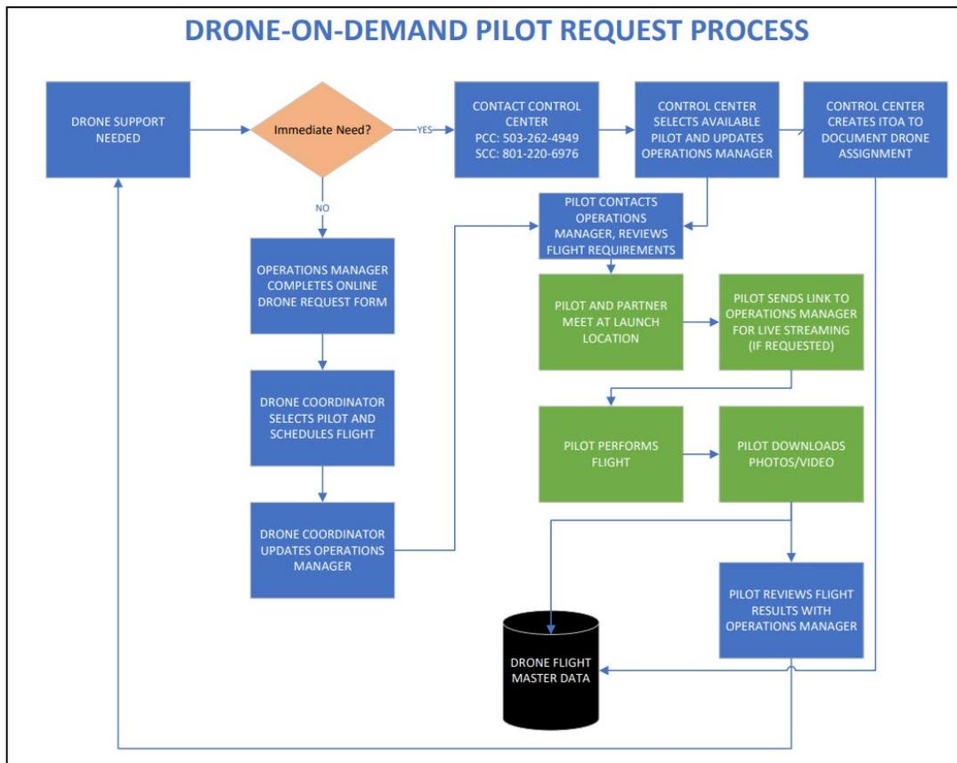
Figure 8-7: Drone on Demand Inspections of Transmission Electric Lines and Equipment Workflow
