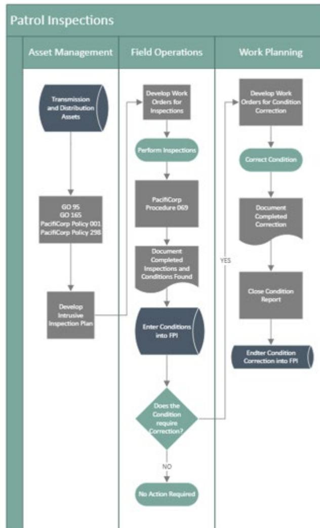
Figure 8-1: Patrol Inspections of Transmission and Distribution Electric Lines and Equipment Workflow
