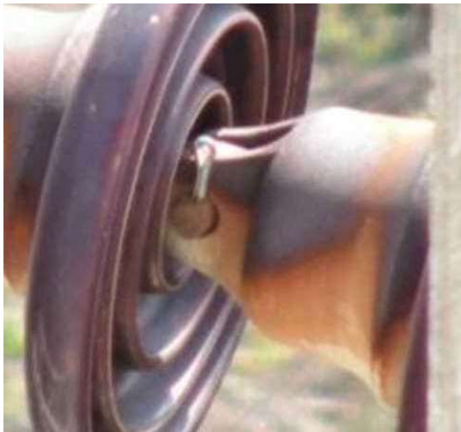
Figure 2–3: P2 (Pin Cotter: Backing Out Cotter Key > Seated Pin > Deadend Assembly > P2)
