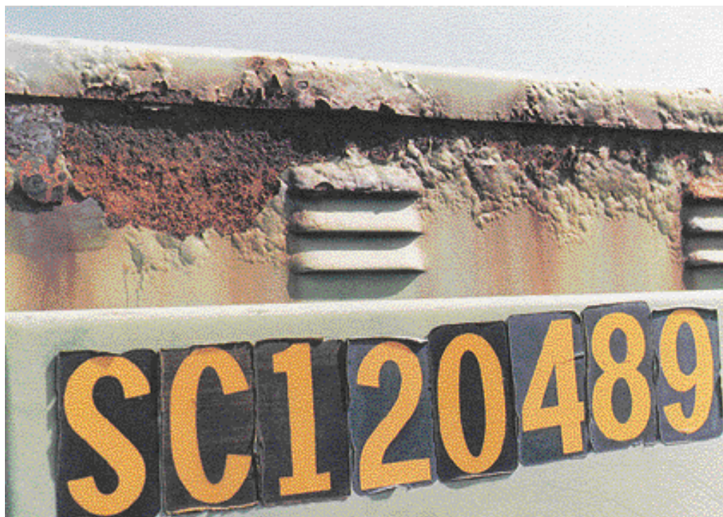
Figure 6–6: Pitting Exceeding One-Quarter Depth of Wall Thickness
