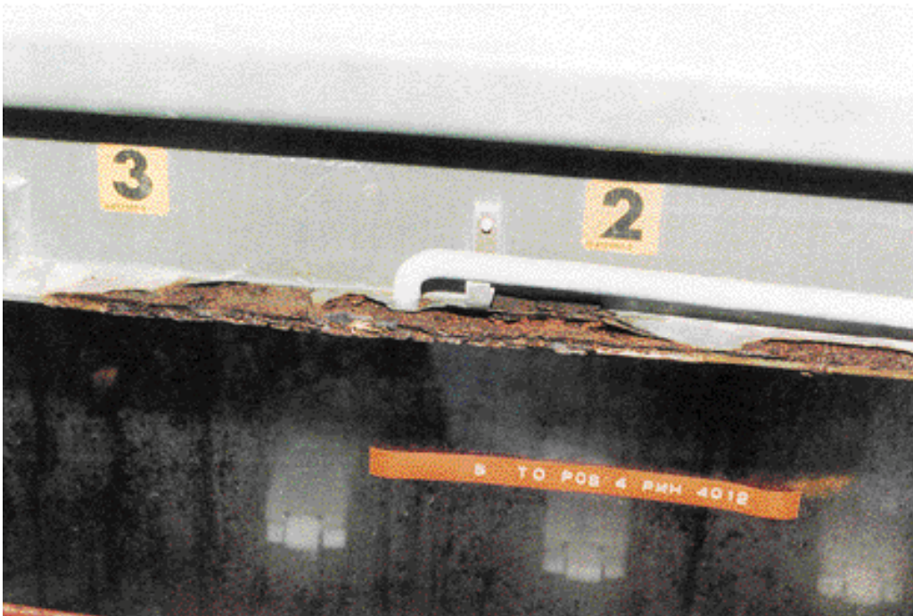
Figure 6–15: Loss of Metal
