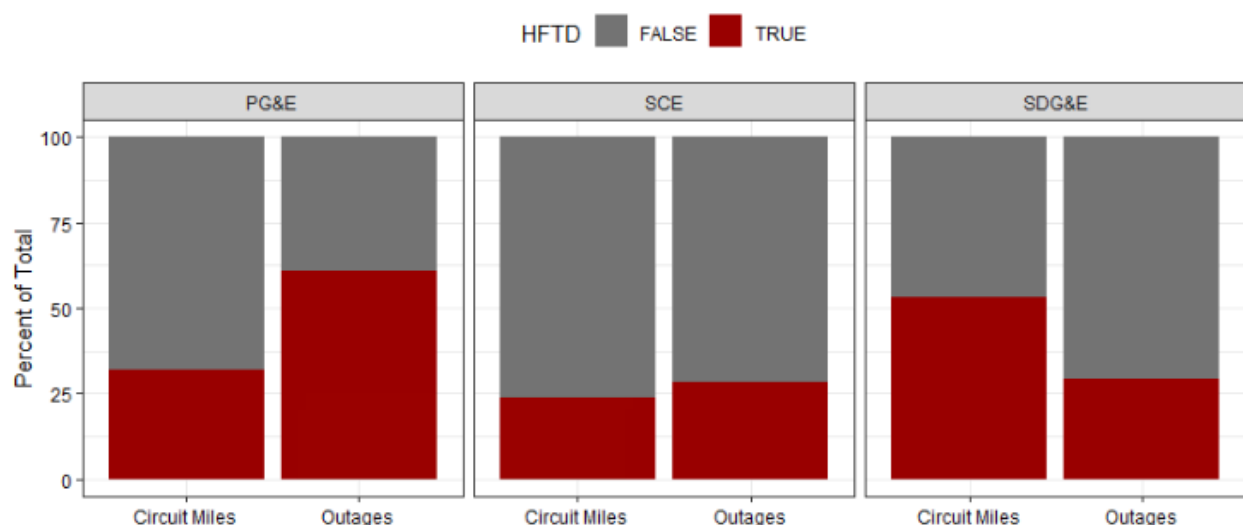
Figure 3-5. Comparison of the proportion of outages from the analysis subset observed in high fire threat district (HFTD) and the proportion of primary overhead circuit miles found in HFTD for each utility.
