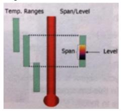
level is the mid point temperature of those numbers. Manually adjusting Span and Level in order to produce a thermogram where the colors are spread over the object of interest, so you can see fine thermal detail and identify thermal gradients.
