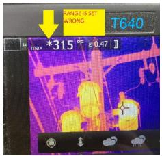
**Distance:** These cameras are calibrated to measure temperatures within a certain distance depending on camera type and FOV of the lens. Do not use the zoom because it makes the pixels bigger and this will distort the image. To accurately read temperatures the radial has to be completely filled with the object of interest. Adding a telescopic lens will measure smaller targets effectively.
