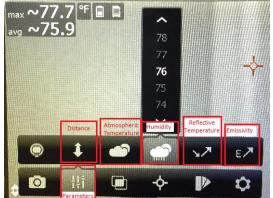
**Temperature:** There are two different temperatures units that can be used, Celsius or Fahrenheit. Check the camera is set to the correct temperature unit before starting.
