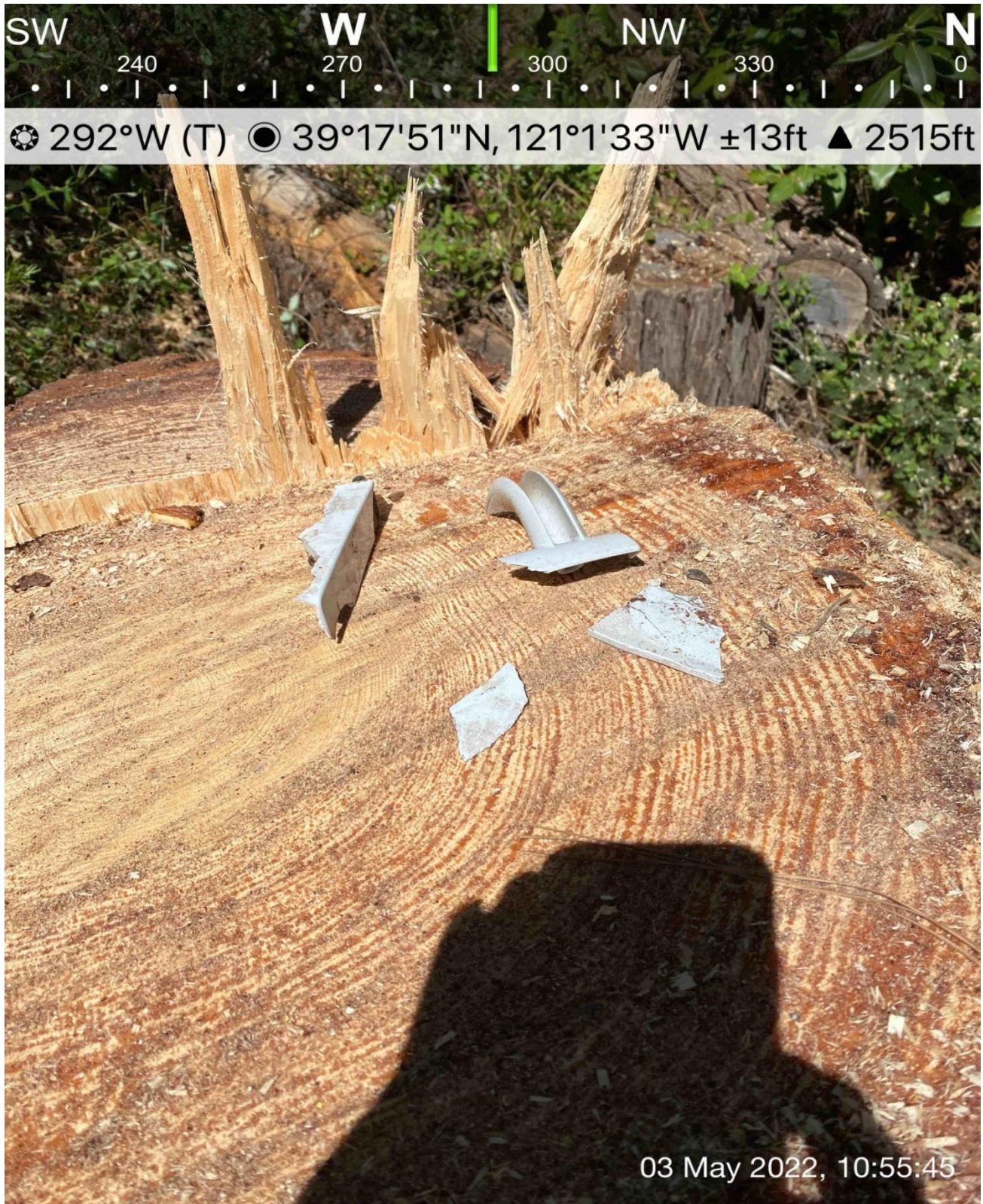
Figure 12 Photo taken by VM team showing broken chainsaw parts on the tree stump.
