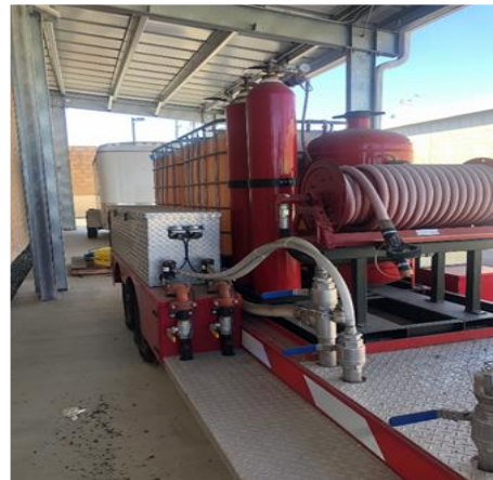
Figure 23 - Foam Trailer, bumper pull lines, & Purple K system with reel line
