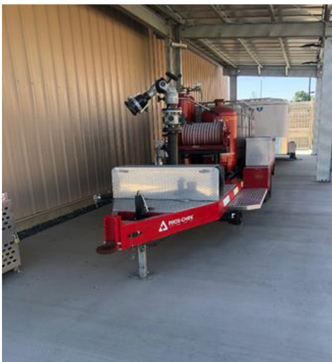
Figure 24 - Foam trailer with foam nozzle
