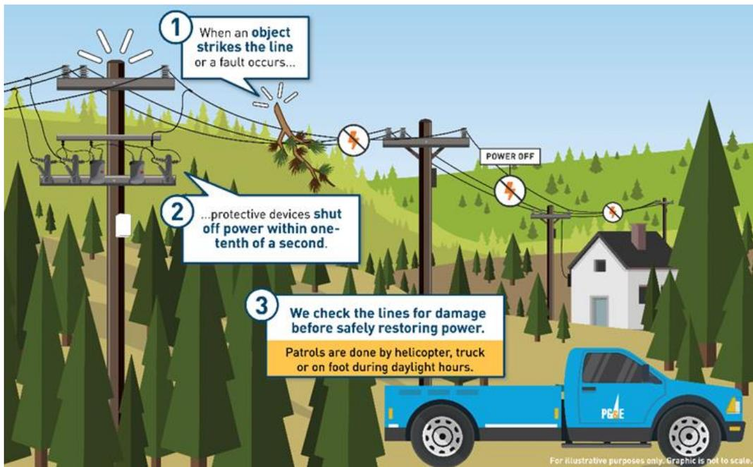
EPSS is a protective technology that allows line protection devices, such as line reclosers, to address faults of varying magnitude and rapidly de-energize the line. These faults may occur due to vegetation striking a line, animal interference, third-party interference (e.g., a vehicle hitting a line) or equipment failure.
