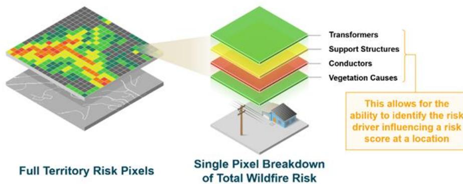
WDRM v3 composites can be built to support specific mitigation strategies. We use the WDRM to support our system hardening, support structures, and transformer mitigations. [Table PG&E-6.2.2-3](#) below shows how compositing has been done for Vegetation Management and System Hardening.
