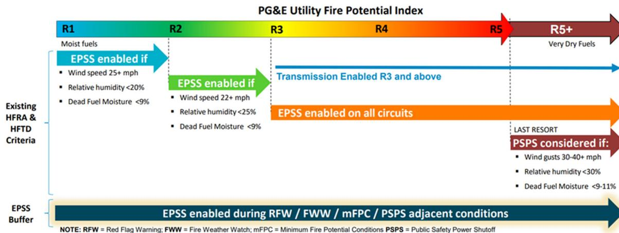
We review multiple meteorological models on a daily basis that indicate—at the individual circuit level—which circuits are forecast to meet EPSS enablement criteria each day. This informs whether circuits need to be enabled for safety or can be disabled.
