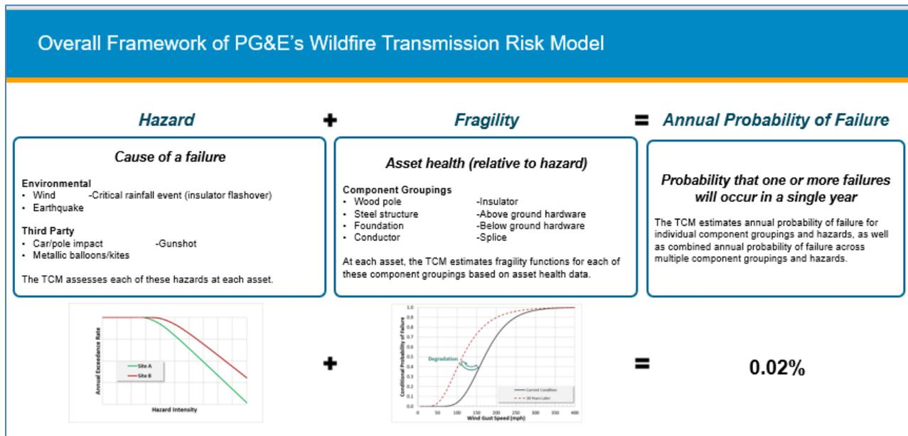
Particularly for machine learning models, risk driver event data enables us to produce more granular sub-models. Due to this, both the nature and location of the failure event is needed to best represent the risk driver that is the objective function of a machine learning model.
