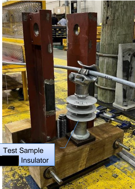
Figure 4-2: Clamp Slip Test Setup
