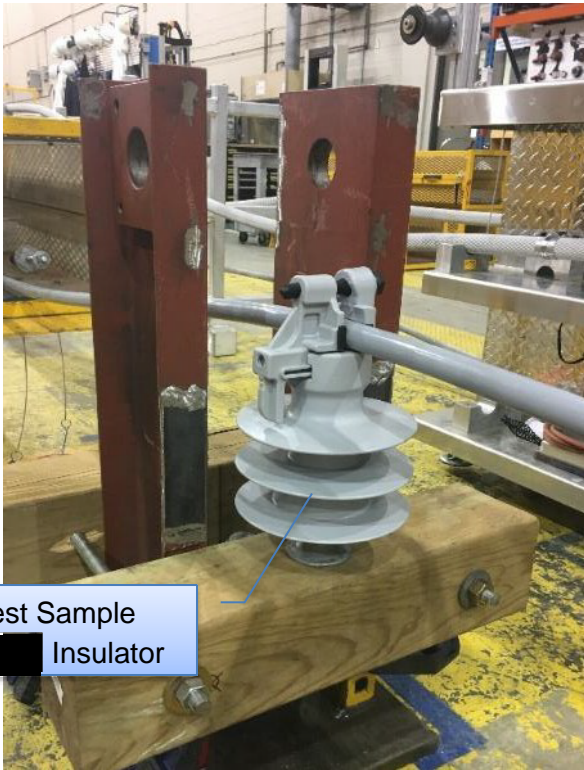
Figure 4-2: Clamp Slip Test Setup
