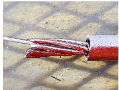
Figure 6-6: Sample 1.1.2 after test (conductor failed at South end of splice)
