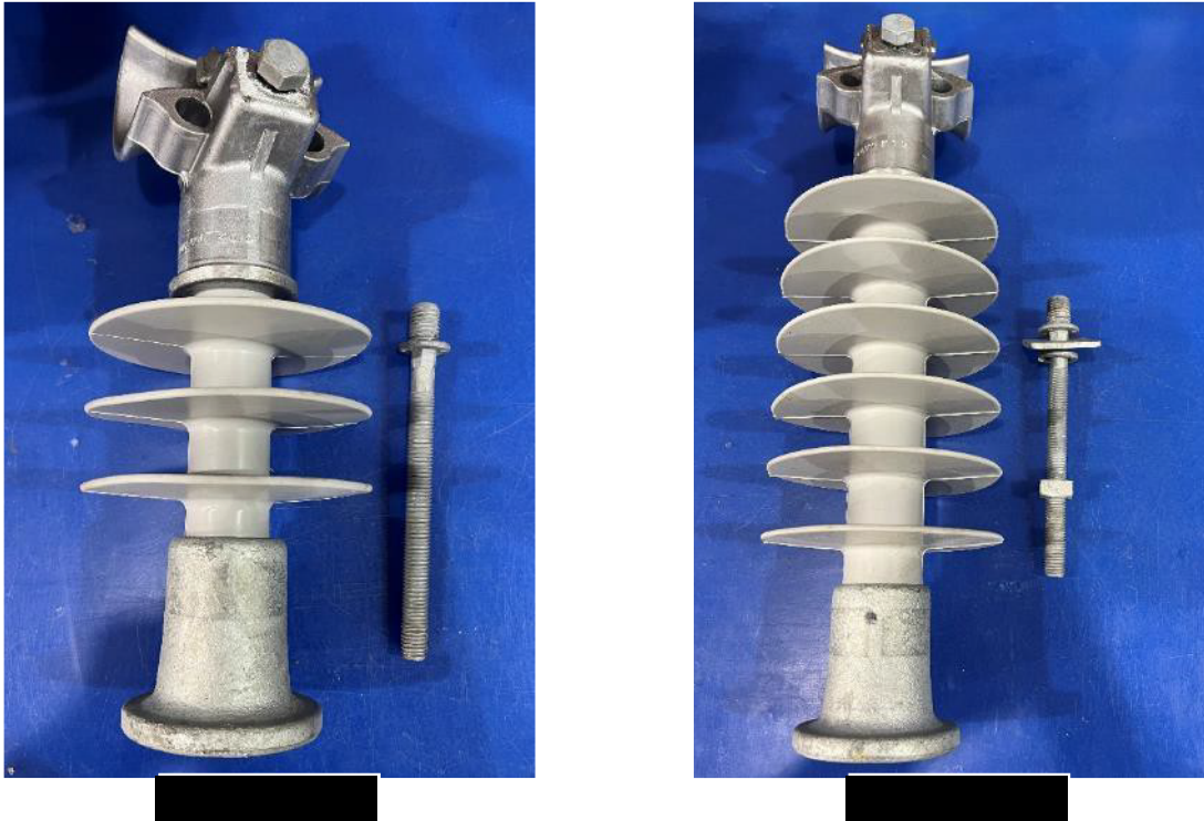
Figure 6-11: [REDACTED] - Typical Insulator and Pin Condition after Slip Test (no damage)
