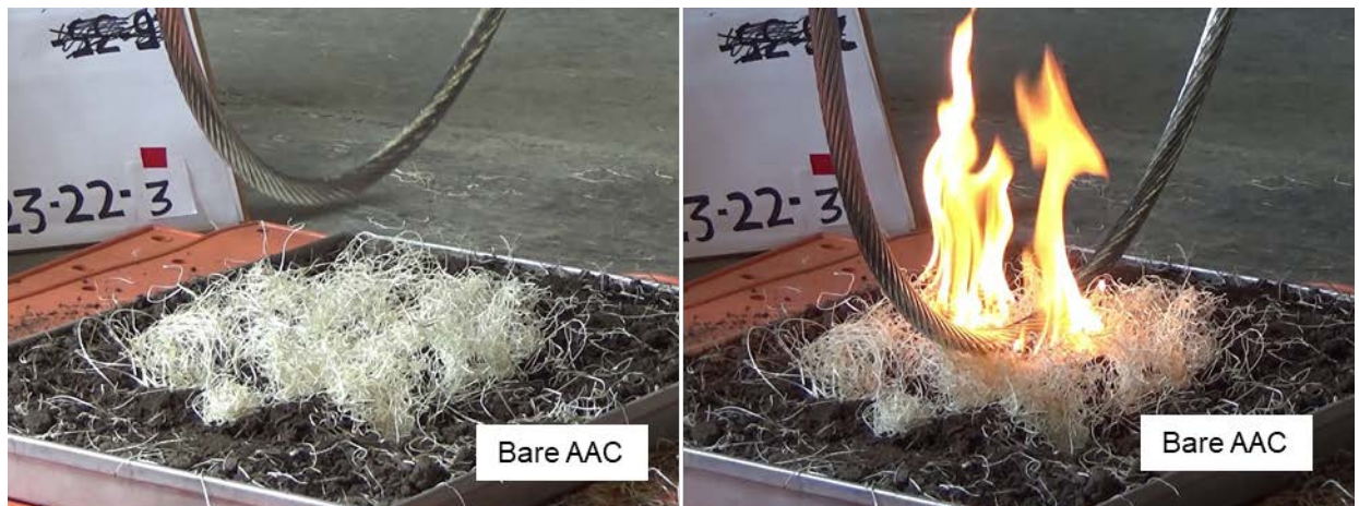
Figure B2. Simulated wire-down test of a bare AAC demonstrating the potential for ignition of the dry brush.
