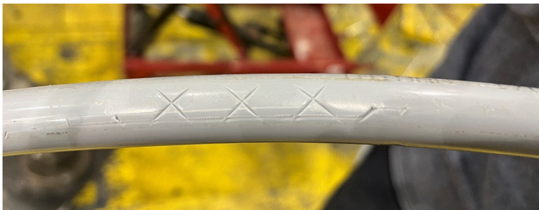
Figure 6-24: Sample 3.4.3 - 15 kV, 1/0 AWG ACSR Condition after Test
