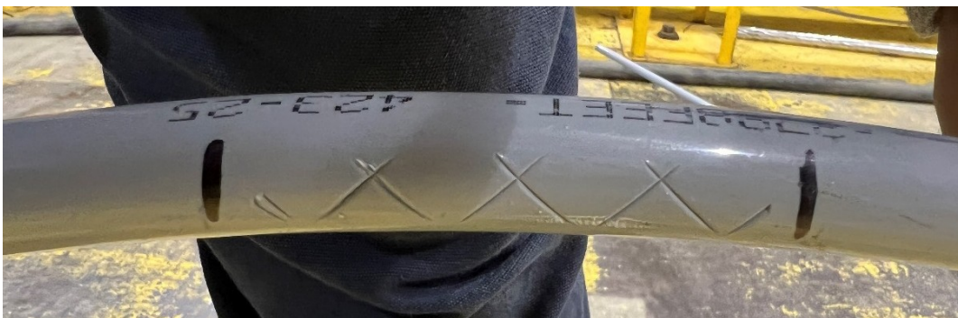
Figure 6-12: Sample 3.1.3 - 17 kV, 1/0 AWG ACSR Condition after Test
