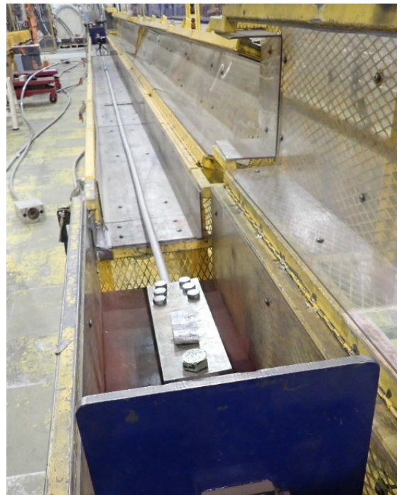
Figure 4-2: Maximum Load Test - Typical Setup
