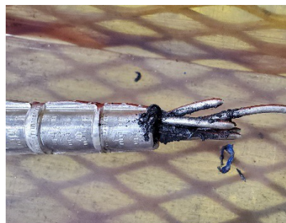
Figure 6-6: Sample 1.1.2 after test (conductor failed at South end of splice)
