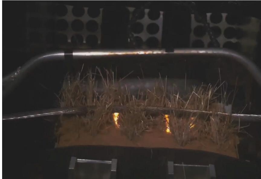
Figure 1-2. Test with REFCL Technology Enabled 2
