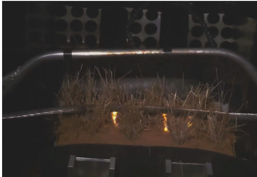
Figure 1-2. Test with REFCL Technology Enabled 2
