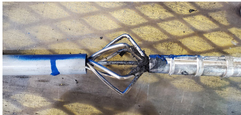
Figure 6-5: Sample 1.1.1 after test (conductor failed at South end of splice)
