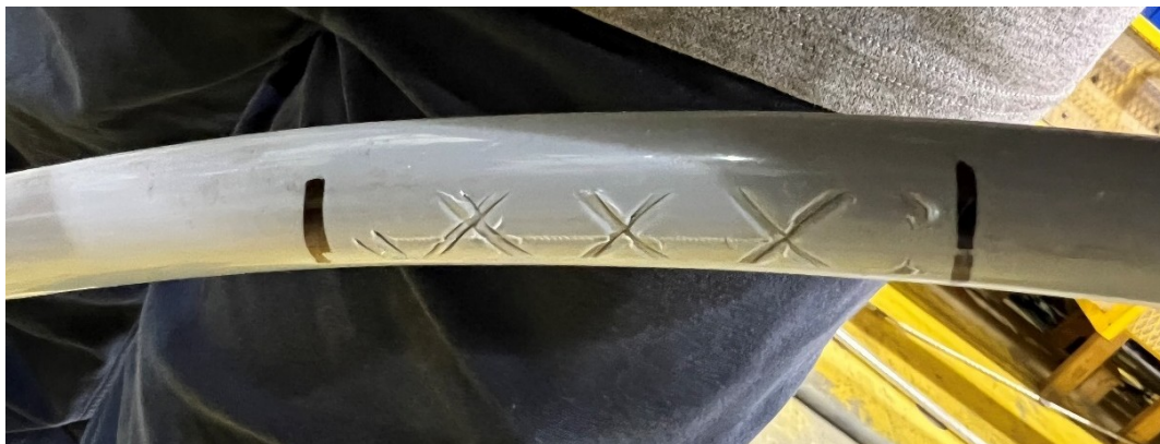
Figure 6-10: Sample 3.1.2 - 17 kV, 1/0 AWG ACSR Condition after Test
