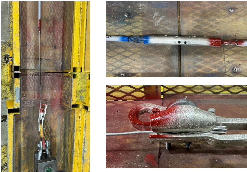
Figure 6-16: Sample 1.4.3 after test
