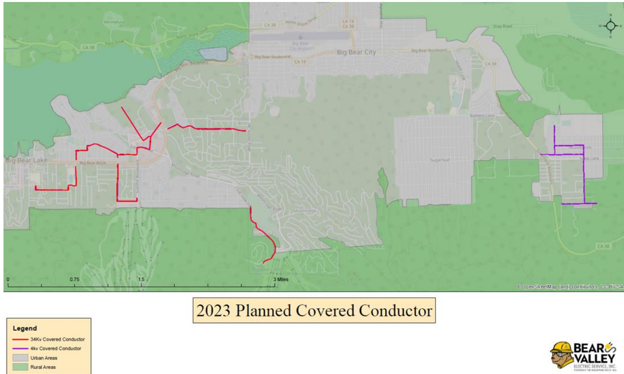
Figure 8-1 2023 Planned Covered Conductor Installation Location
