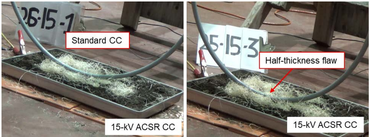
Figure B5. (Left) Simulated wire-down test of a 15-kV ACSR CC. No ignition was observed after three tests. (Right) Simulated wire-down test of a 15-kV ACSR CC with a half-thickness flaw. No ignition was observed after three tests.
