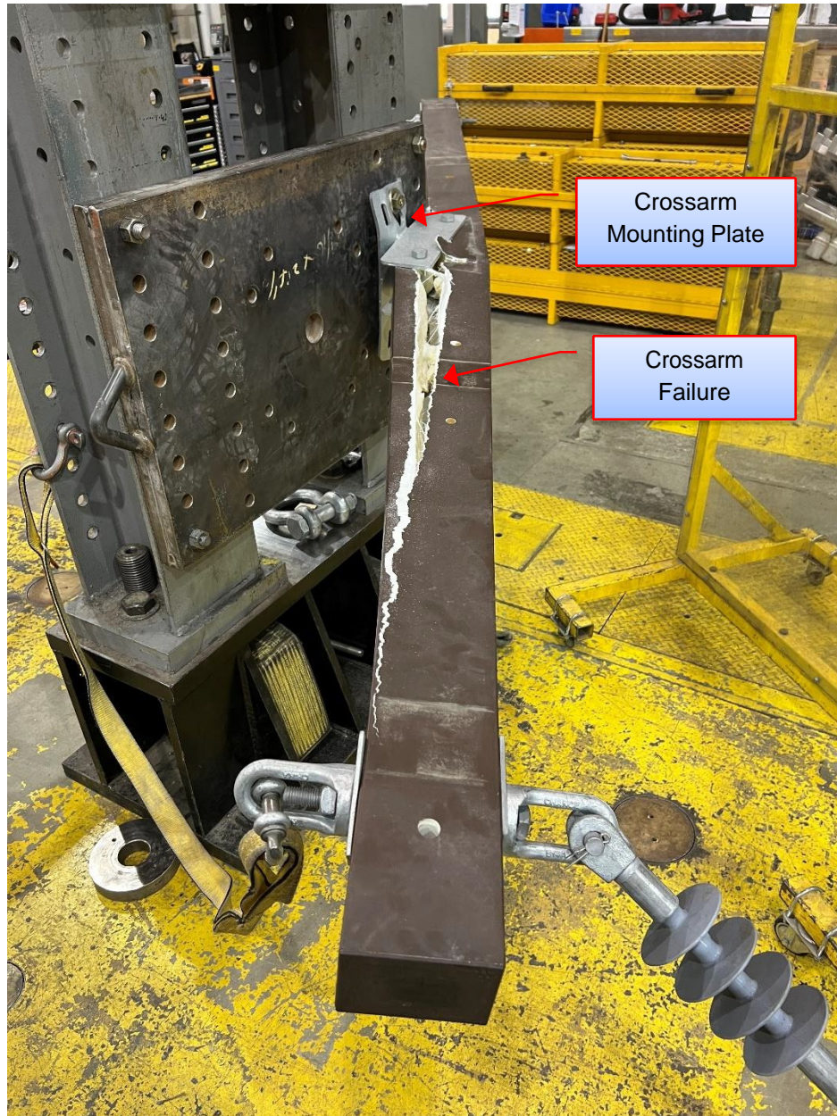
Figure 6-25: Sample 7.1 – Failure Location
