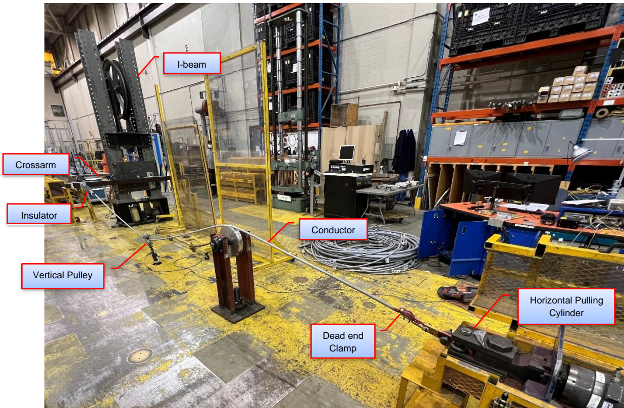
Figure 4-3: Full Mock-up: Picture of the Setup
