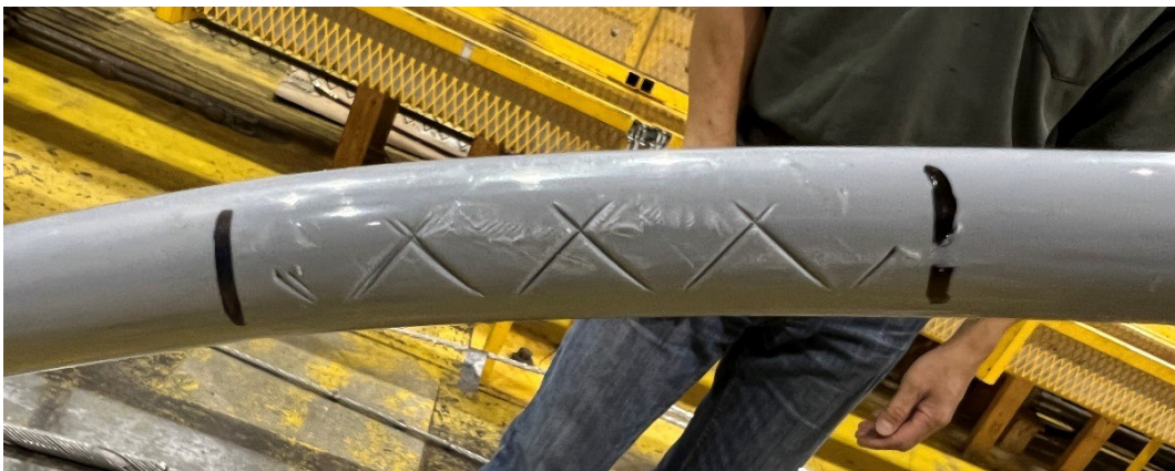
Figure 6-8: Sample 3.1.1 - 17 kV, 1/0 AWG ACSR Condition after Test
