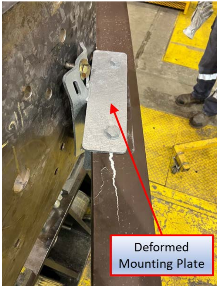
Figure E5. A representative post-test image showing typical deformation of the cross-arm mounting plate.
