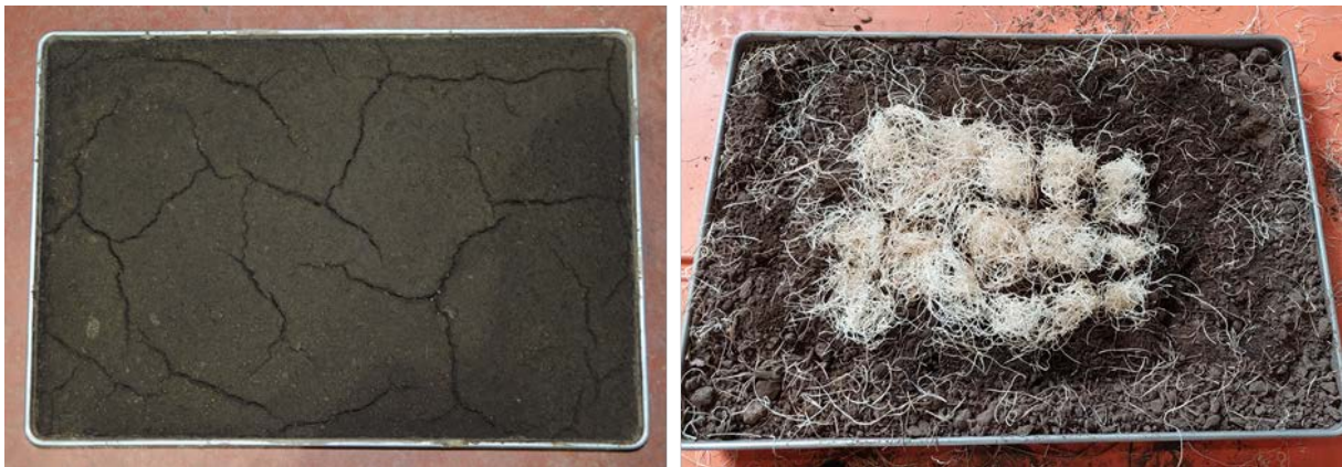
Figure 21. Example of simulated California soil and fuel bed used in wire-down testing.
