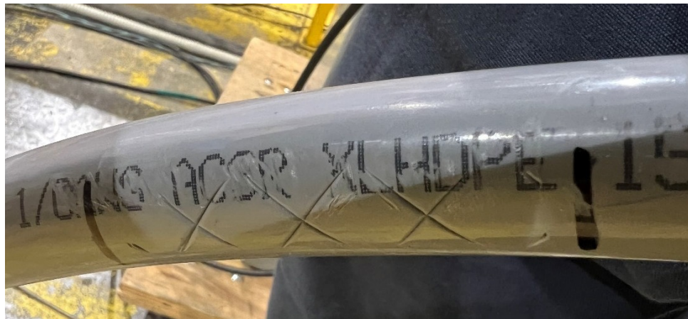
Figure 6-15: Sample 3.2.2 - 35 kV, 1/0 AWG ACSR Condition after Test
