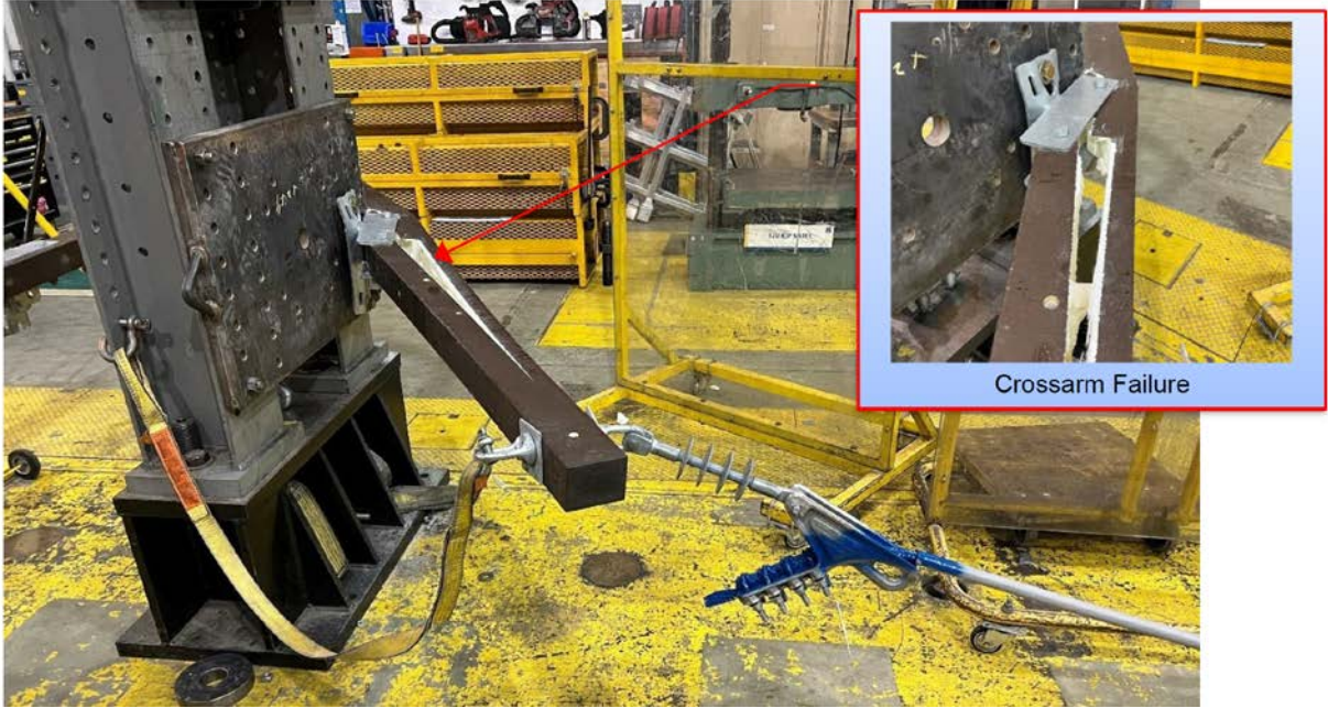
Figure E4. A representative post-test image showing splitting and failure of the composite cross-arm. 336.4 kcmil ACSR (30/7) with Type C dead-end shown.
