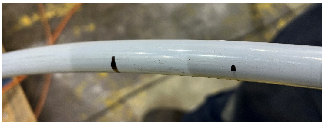
Figure 6-28: Sample 3K.1.2 - 17 kV, 1/0 AWG ACSR Condition after Test
