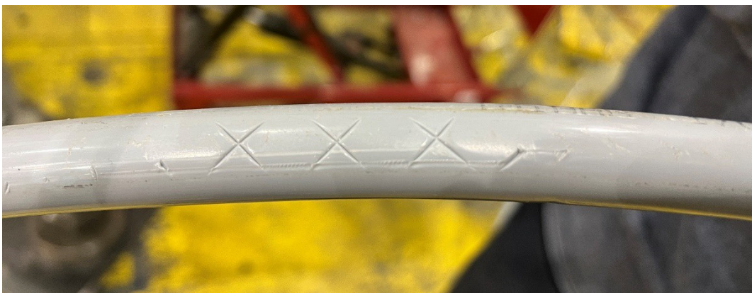
Figure 6-24: Sample 3.4.3 - 15 kV, 1/0 AWG ACSR Condition after Test
