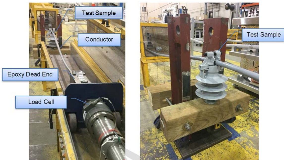
Figure 61. Representative photos of insulator slip test.
