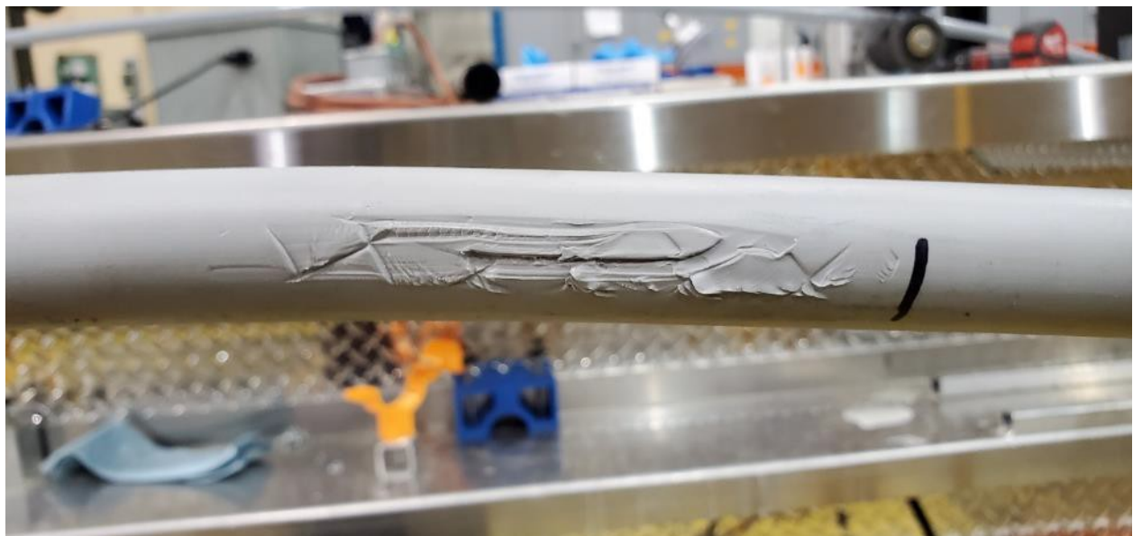
Figure 6-4: [REDACTED] - Typical 397.5 kcmil (22 kV) AAC Conductor Condition after Slip Test
