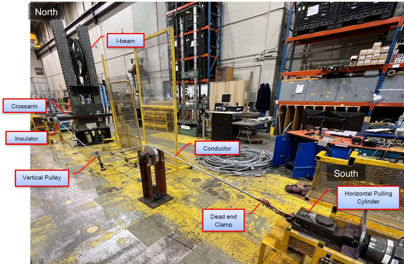
Figure E2. A representative photo of the dead-end tree fall test.
