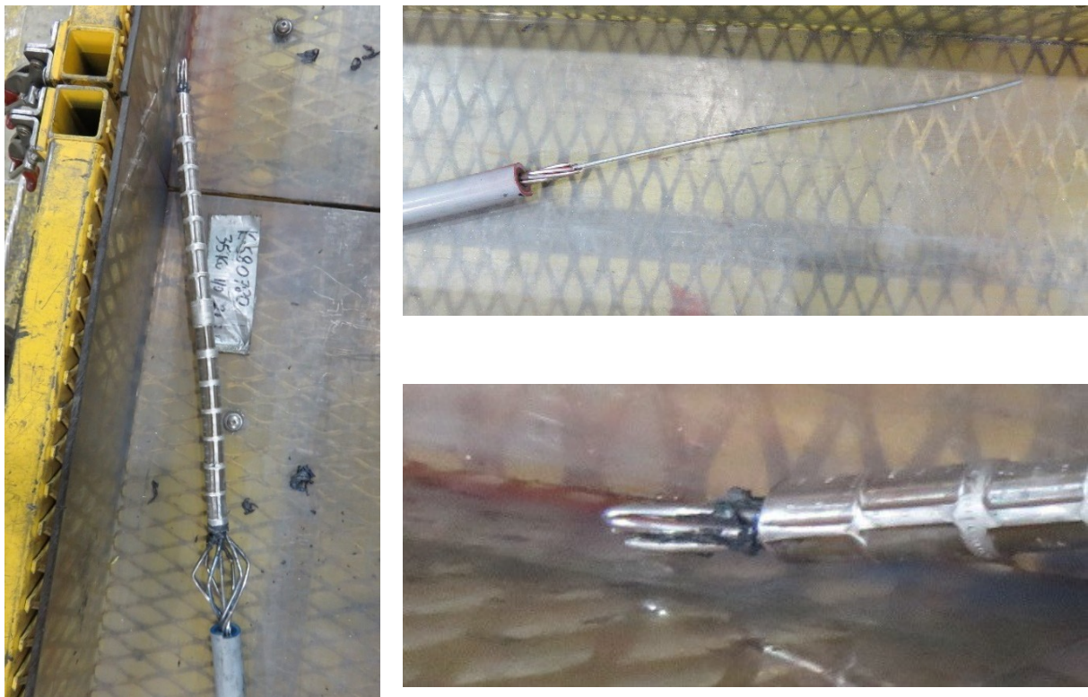
Figure 6-8: Sample 1.2.1 after test (conductor failed at North end of splice)
