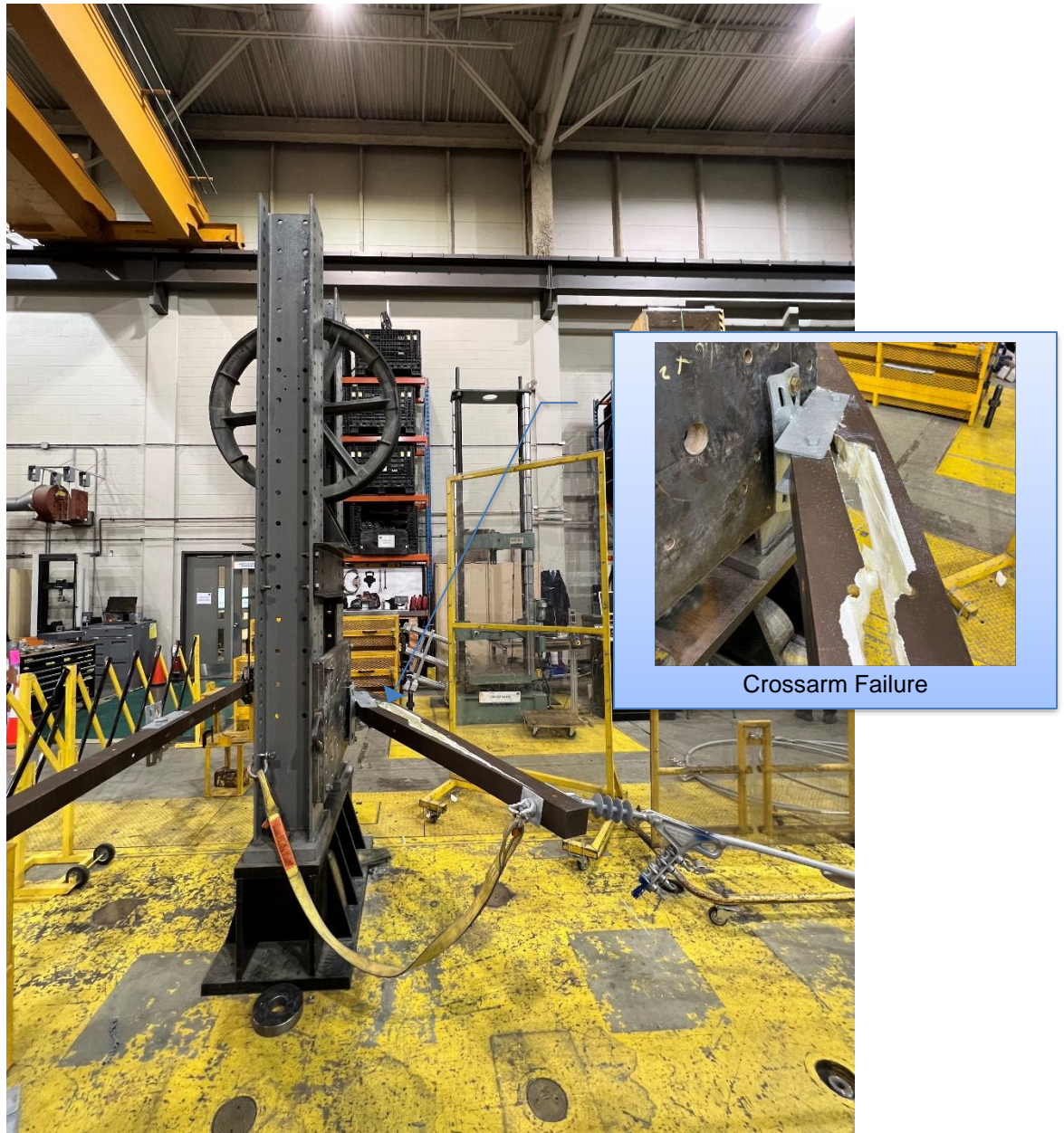
Figure 6-22: Sample 6.1 – Failure Location
