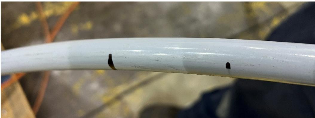
**Figure 6-34: Sample 3K.1.3 - 17 kV, 1/0 AWG ACSR Condition after Test**
