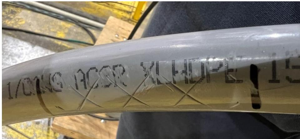
Figure 6-15: Sample 3.2.2 - 35 kV, 1/0 AWG ACSR Condition after Test
