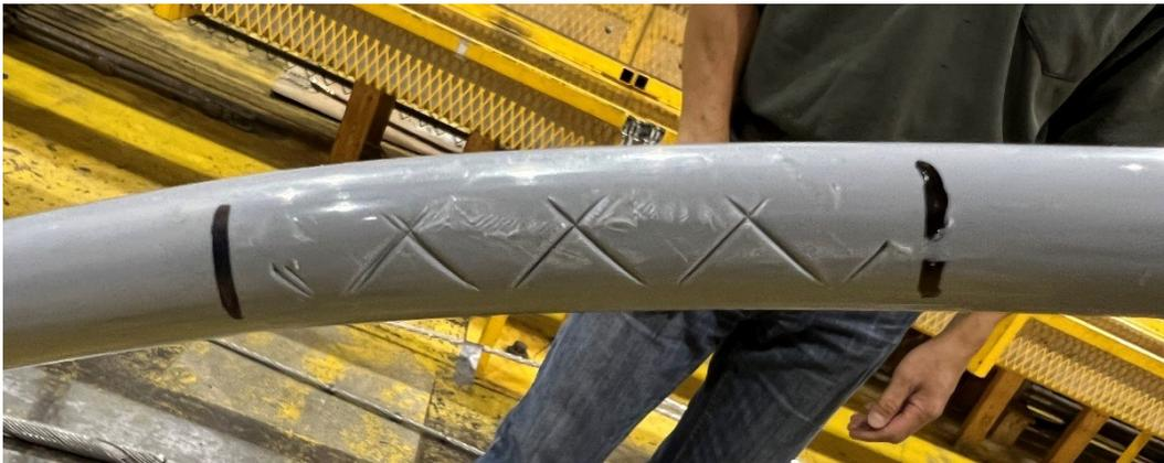
**Figure 6-8: Sample 3.1.1 - 17 kV, 1/0 AWG ACSR Condition after Test**
