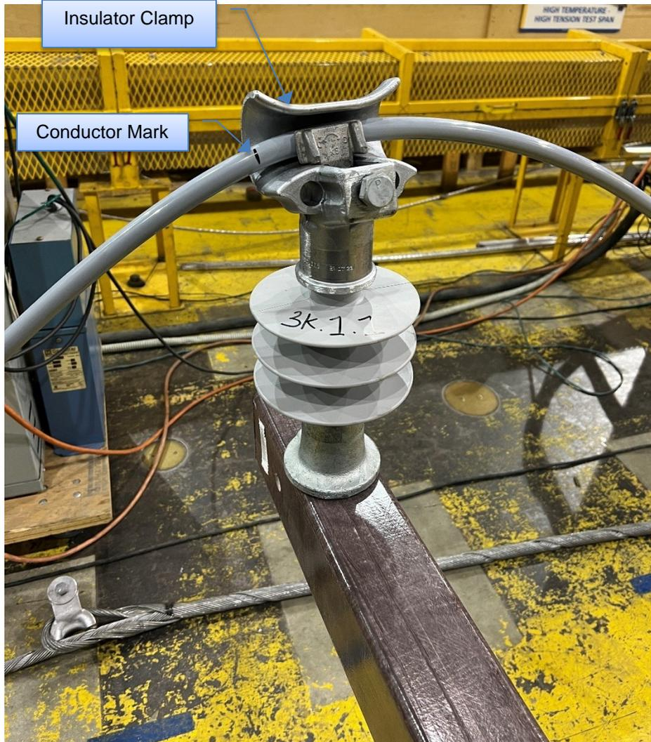
Figure 6-25: Sample 3K.1.1 – Insulator and Cross-arm Condition after Test
