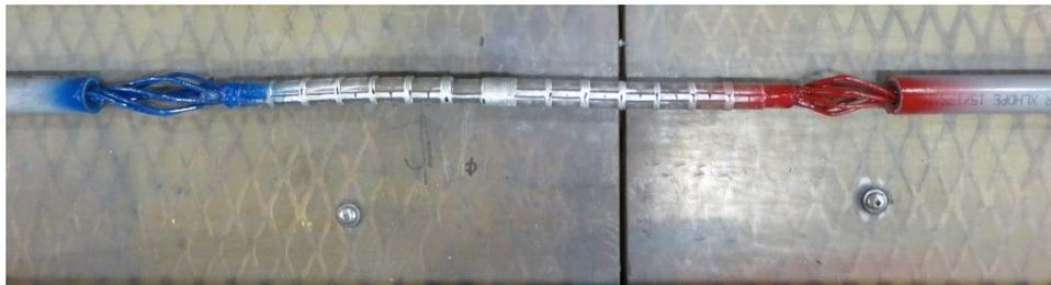
**Figure 3-3: ██████ installed on 35 kV 1/0 AWG, 6/1 ACSR**
