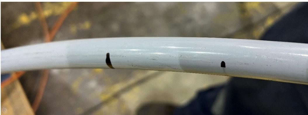
**Figure 6-30: Sample 3K.1.3 - 17 kV, 1/0 AWG ACSR Condition after Test**
