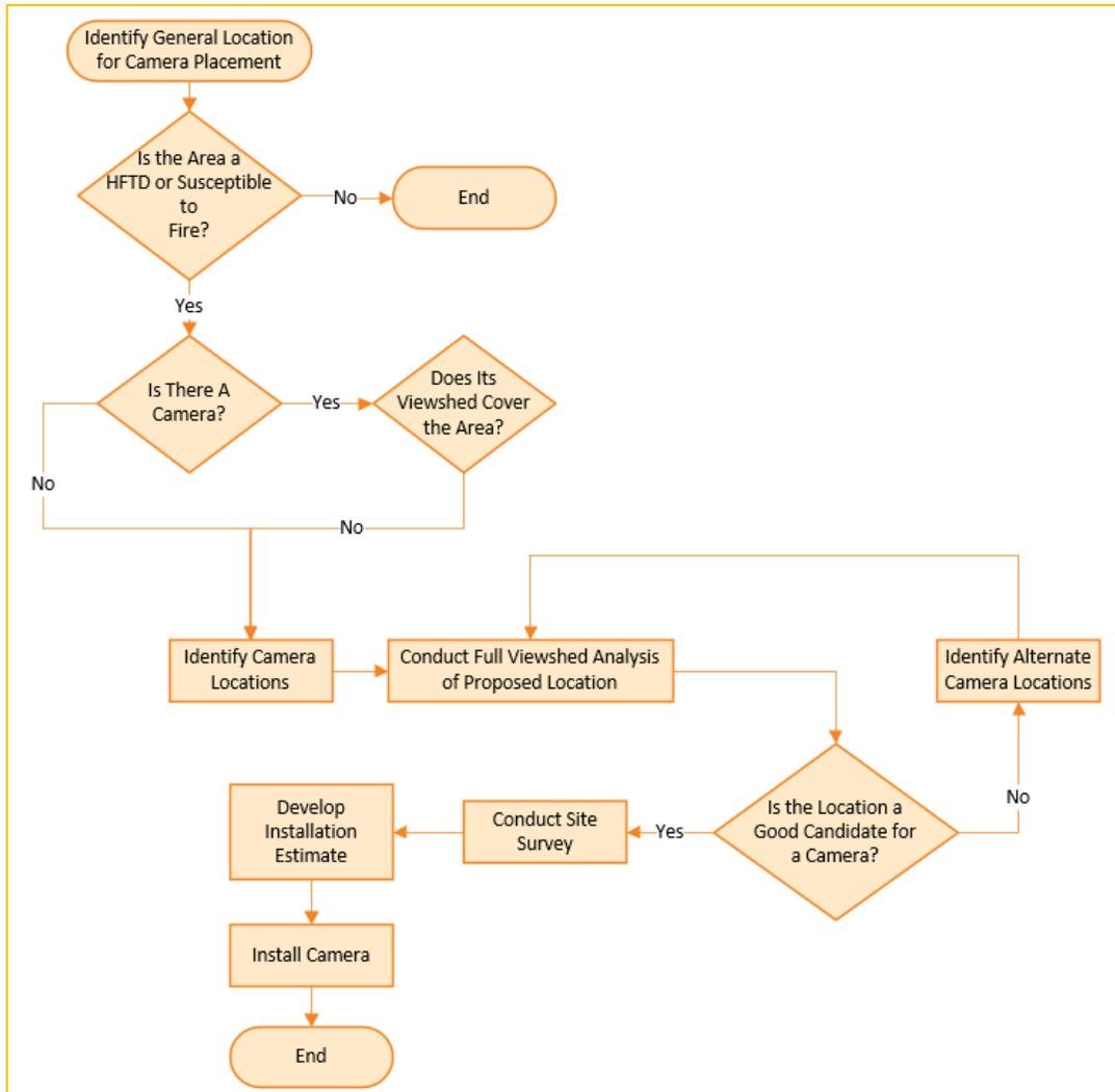
**Figure 8-20 Camera Placement Methodology**
