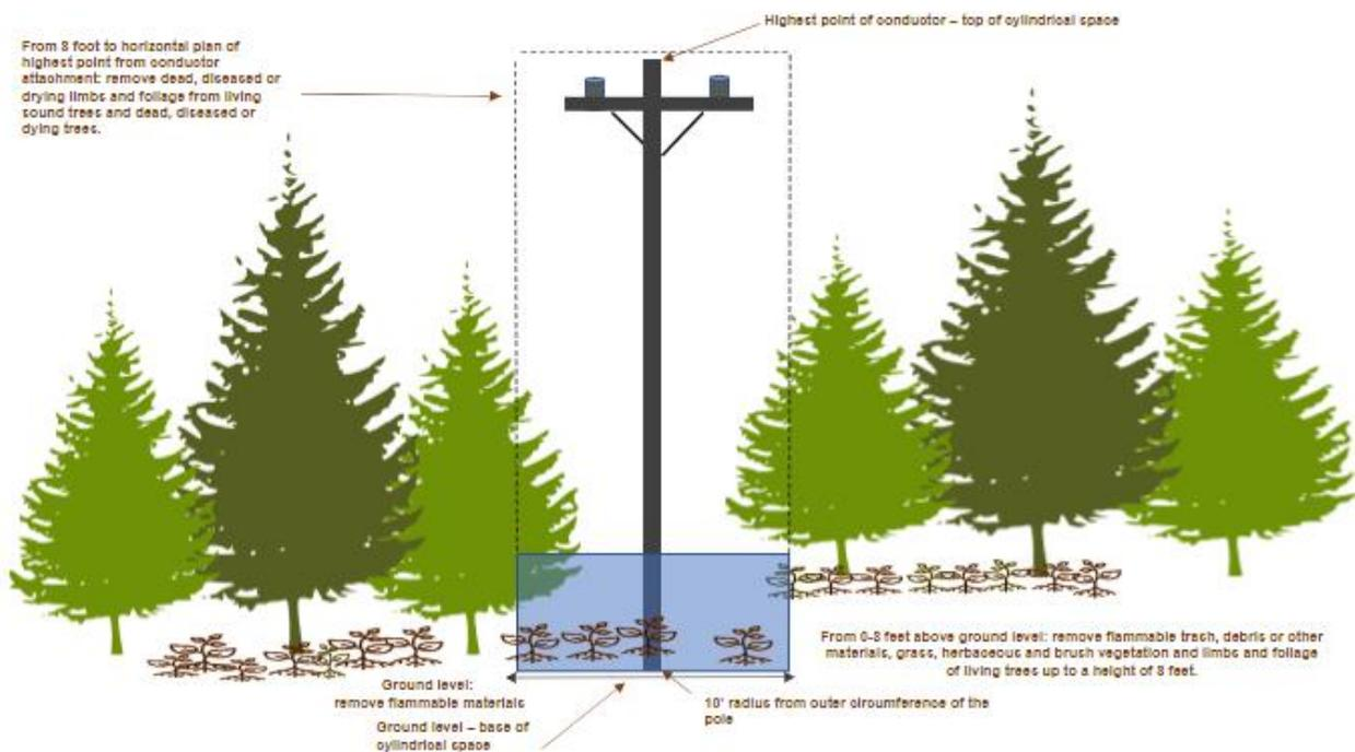
**Figure 8-12 Pole Clearing**
