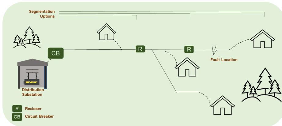
**Figure 8-7: Example of Distribution Circuit with Multiple Reclosers**
