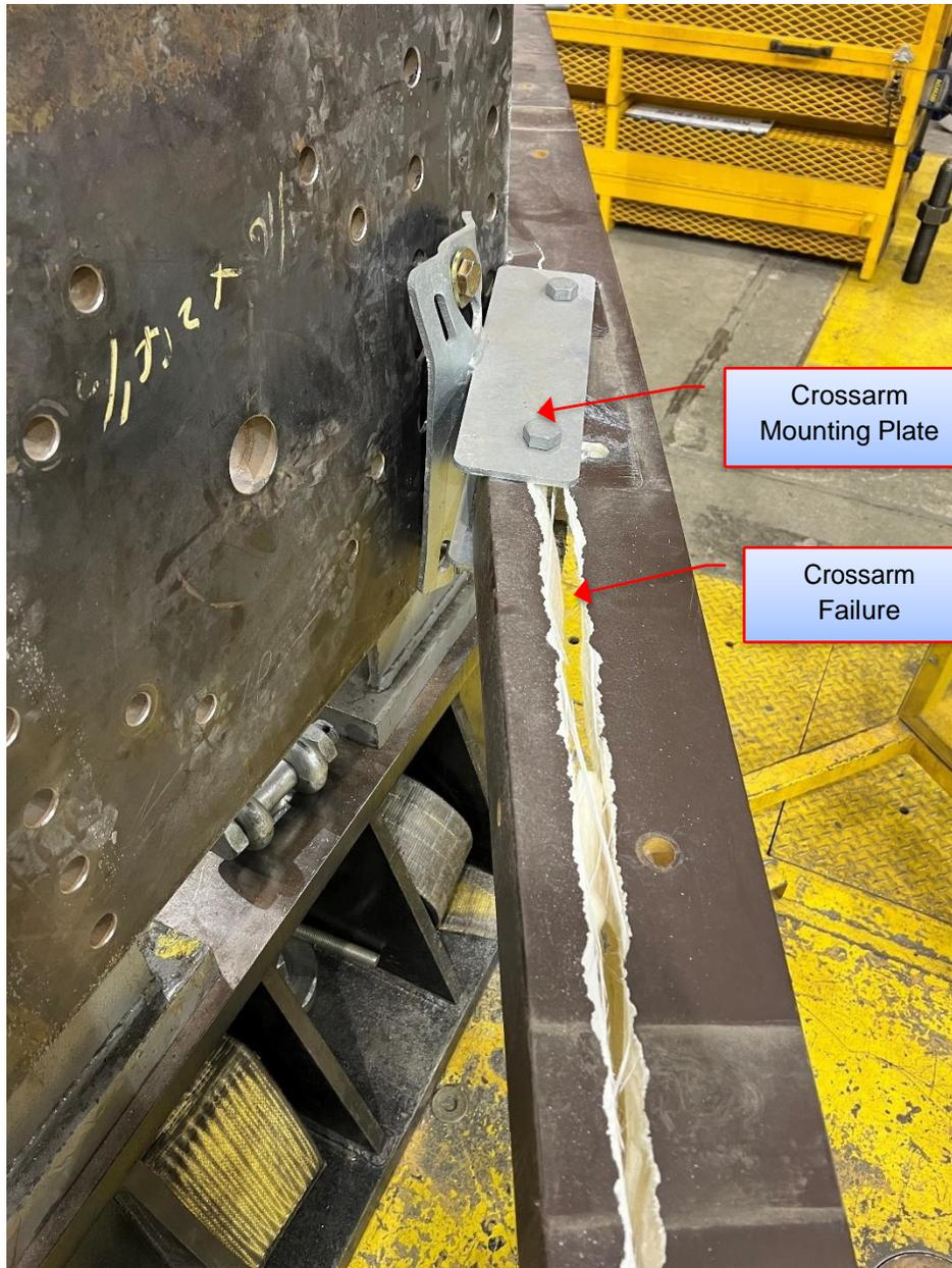
**Figure 6-27: Sample 7.3 – Failure Location**
