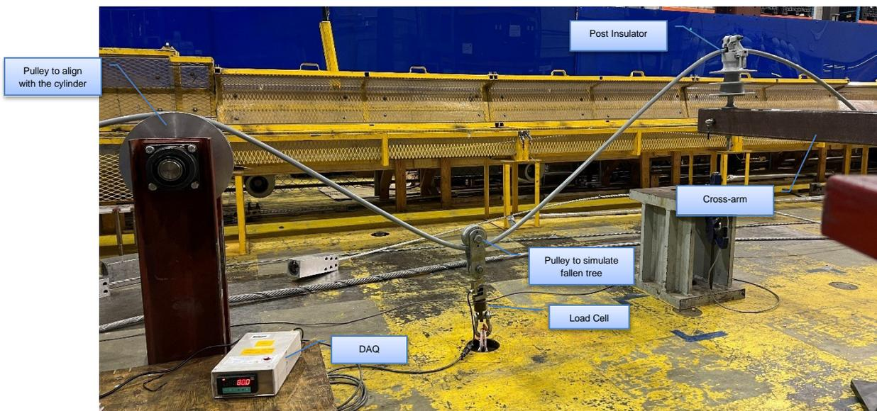
Figure 4-2: Full Mock-up Test - Picture of the Setup
