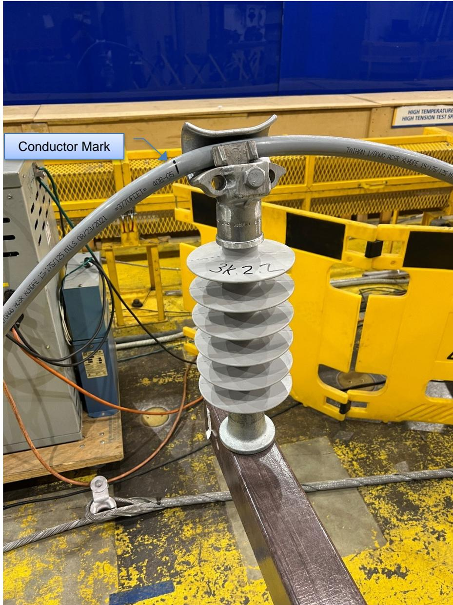
Figure 6-32: Sample 3K.2.2 – Insulator and Cross-arm Condition after Test
