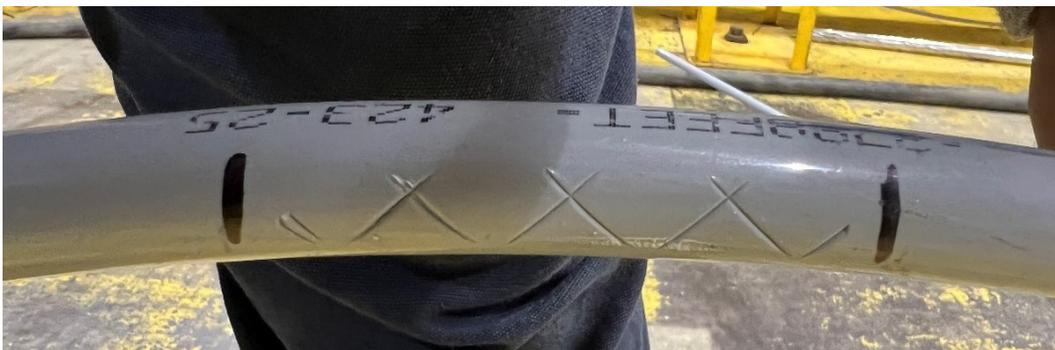
Figure 6-12: Sample 3.1.3 - 17 kV, 1/0 AWG ACSR Condition after Test
