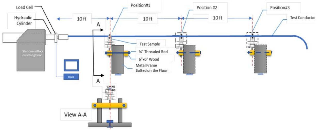
Figure 60. Schematic diagram of insulator slip test.
