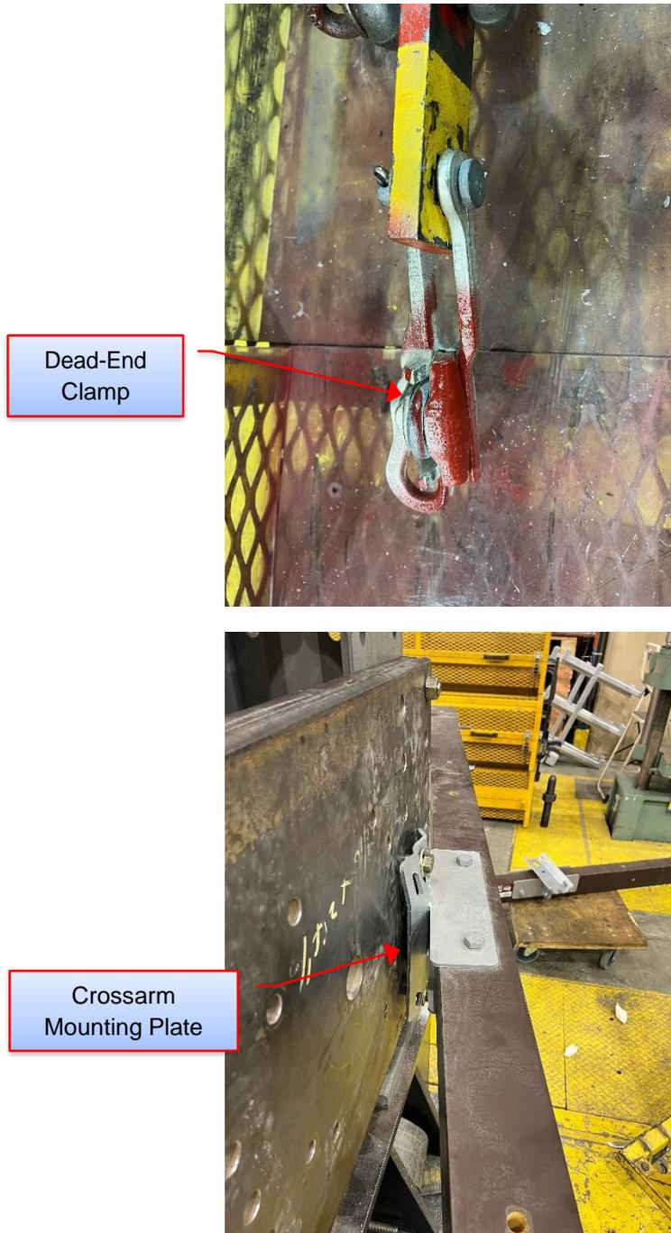
**Figure 6-15: Sample 3.2 – Failure Location**
