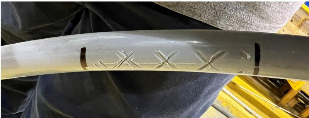
**Figure 6-10: Sample 3.1.2 - 17 kV, 1/0 AWG ACSR Condition after Test**
