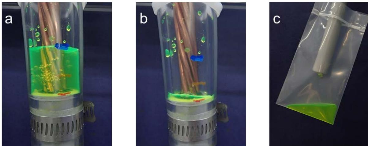
Figure 29. Representative photographs of liquid ingress testing performed on 17-kV copper CCs. (a) Liquid was introduced to the stripped end of a 17-kV copper CC at  $t=0$ . (b-c) After five minutes ( $t=5$ ), the liquid level had dropped significantly at the stripped end (b), and liquid output was observed at the far end of the CC (c).
