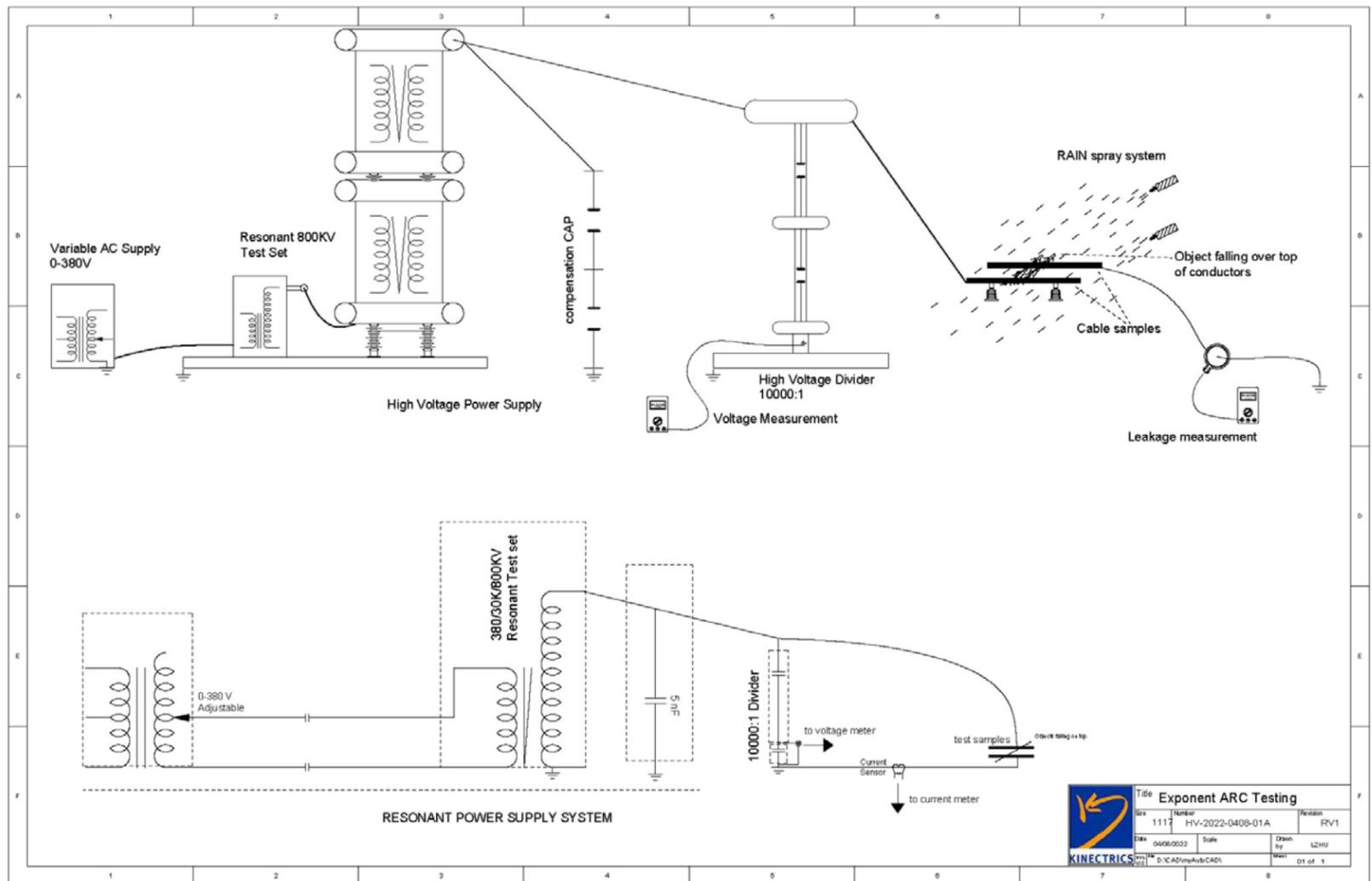
Figure A1. Phase-to-phase contact tests.
