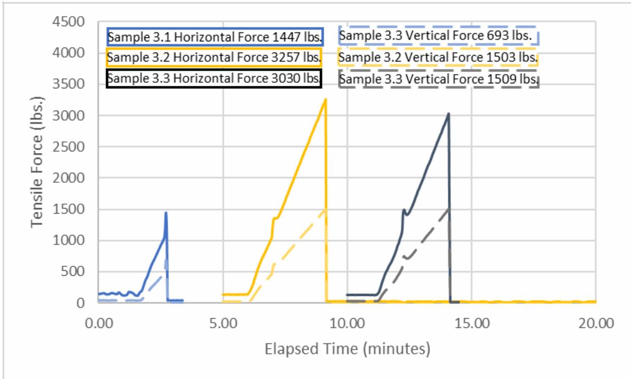
**Figure 6-3: Test Load Profile: 17kV 4/0 AWG, 19 CU Conductor**
