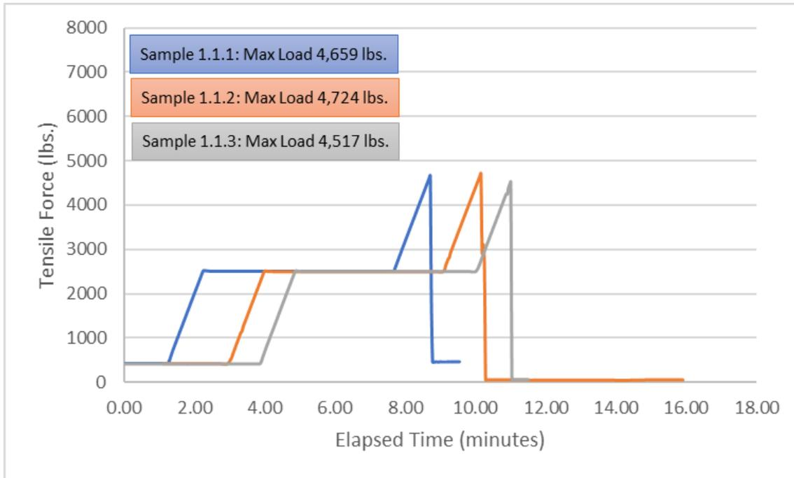
**Figure 6-1: Maximum Load Test – 17 kV, 1/0 AWG ACSR**
