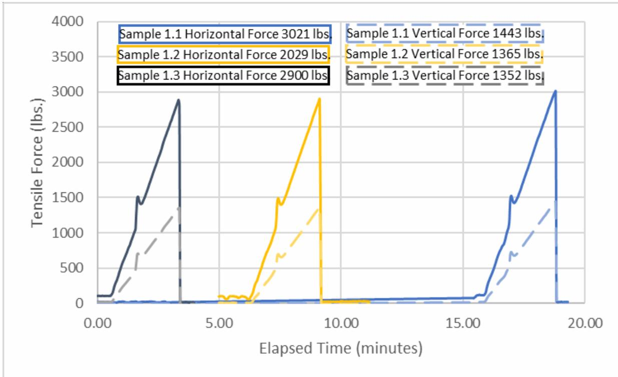
**Figure 6-1: Test Load Profile: 17KV #2 AWG, 7 CU Conductor**
