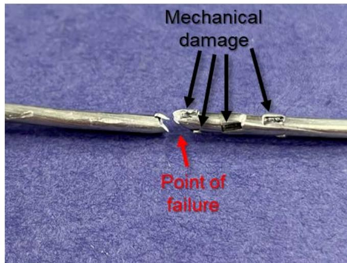
Figure 45. Photograph of a single aluminum strand from a 15-kV ACSR CC with IPC hardware after salt spray exposure and tensile testing. The mechanical damage was caused by the IPC hardware and was unrelated to either the salt spray testing or the tensile testing.
