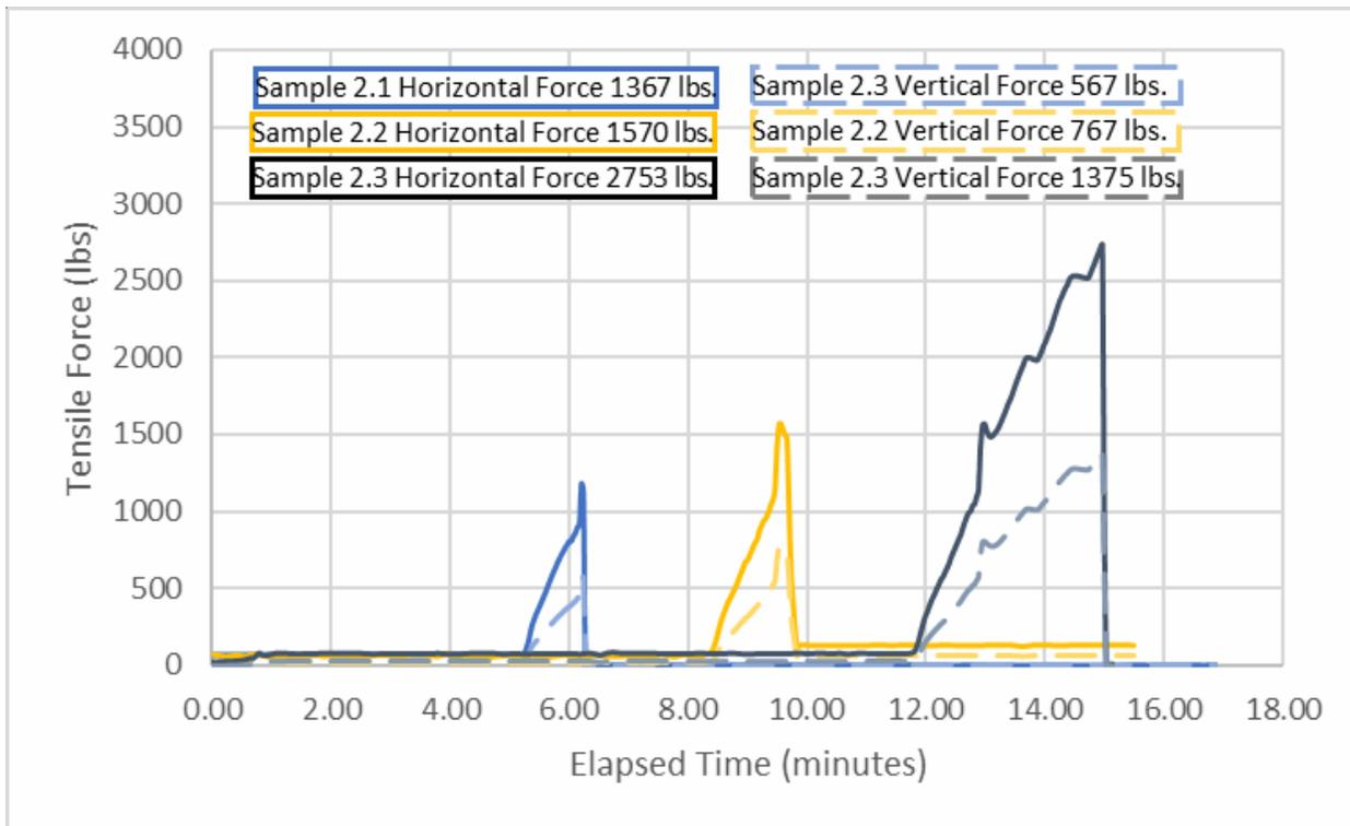
**Figure 6-2: Test Load Profile: 17kV 2/0 AWG, 19 CU Conductor**
