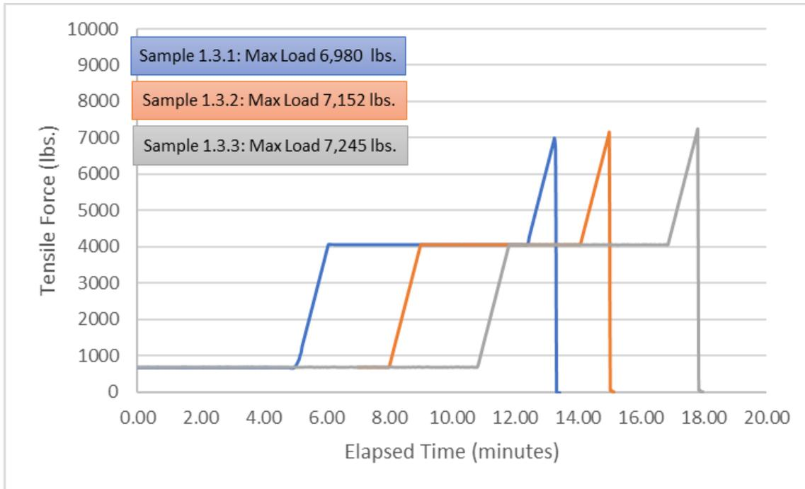
**Figure 6-3: Maximum Load Test – 22 kV, 397.5 kcmil AAC**
