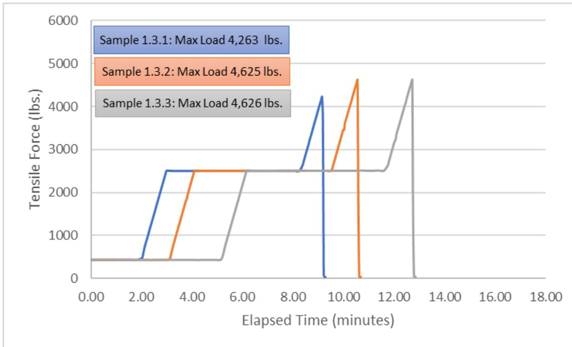
**Figure 6-4: Maximum Load Test – 15 kV, 1/0 AWG ACSR**
