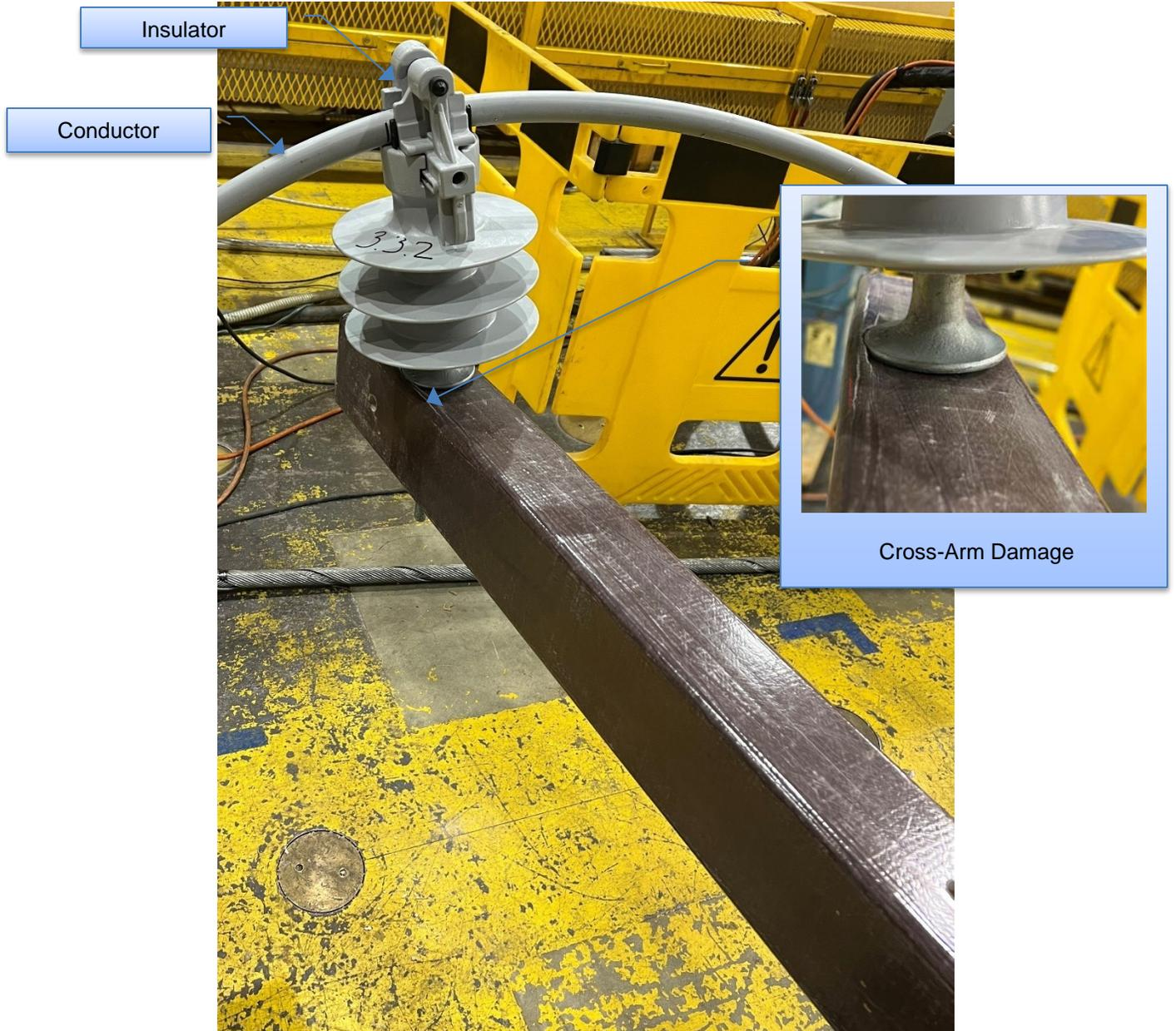
**Figure 6-18: Sample 3.3.2 - Insulator and Cross-arm Condition after Test**
