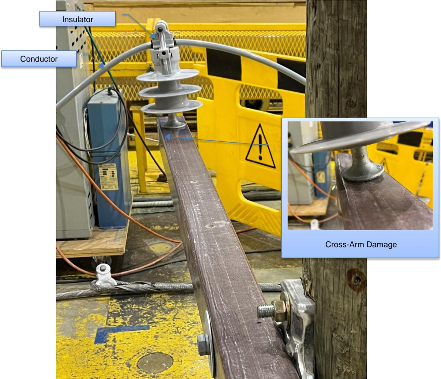
Figure 6-21: Sample 3.4.1 – Insulator and Cross-arm Condition after Test
