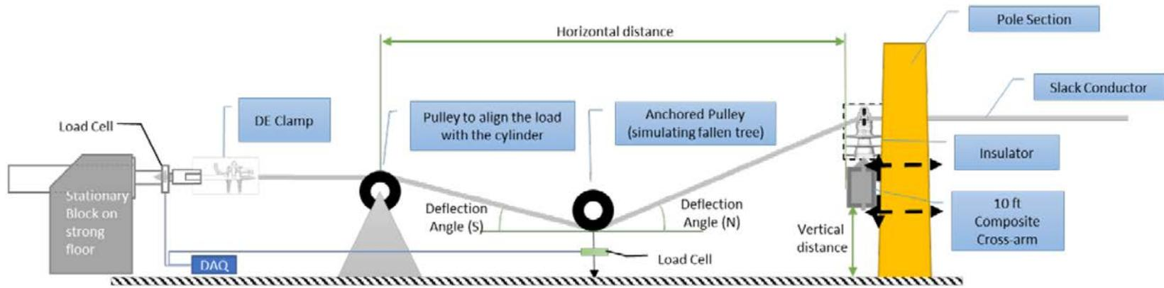
Figure 63. Schematic diagram of the full-system tree-fall test.
