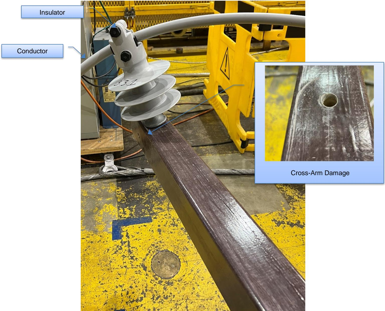
Figure 6-17: Sample 3.3.1 – Insulator and Cross-arm Condition after Test
