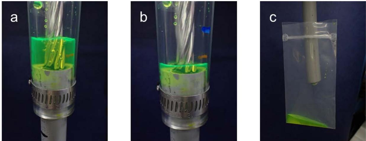
Figure 28. Representative photographs of liquid ingress testing performed on 17-kV ACSR CCs. (a) Liquid was introduced to the stripped end of a 17-kV ACSR CC at  $t=0$ . (b-c) After five minutes, the liquid level had dropped significantly at the stripped end (b), and liquid output was observed at the far end of the CC (c).
