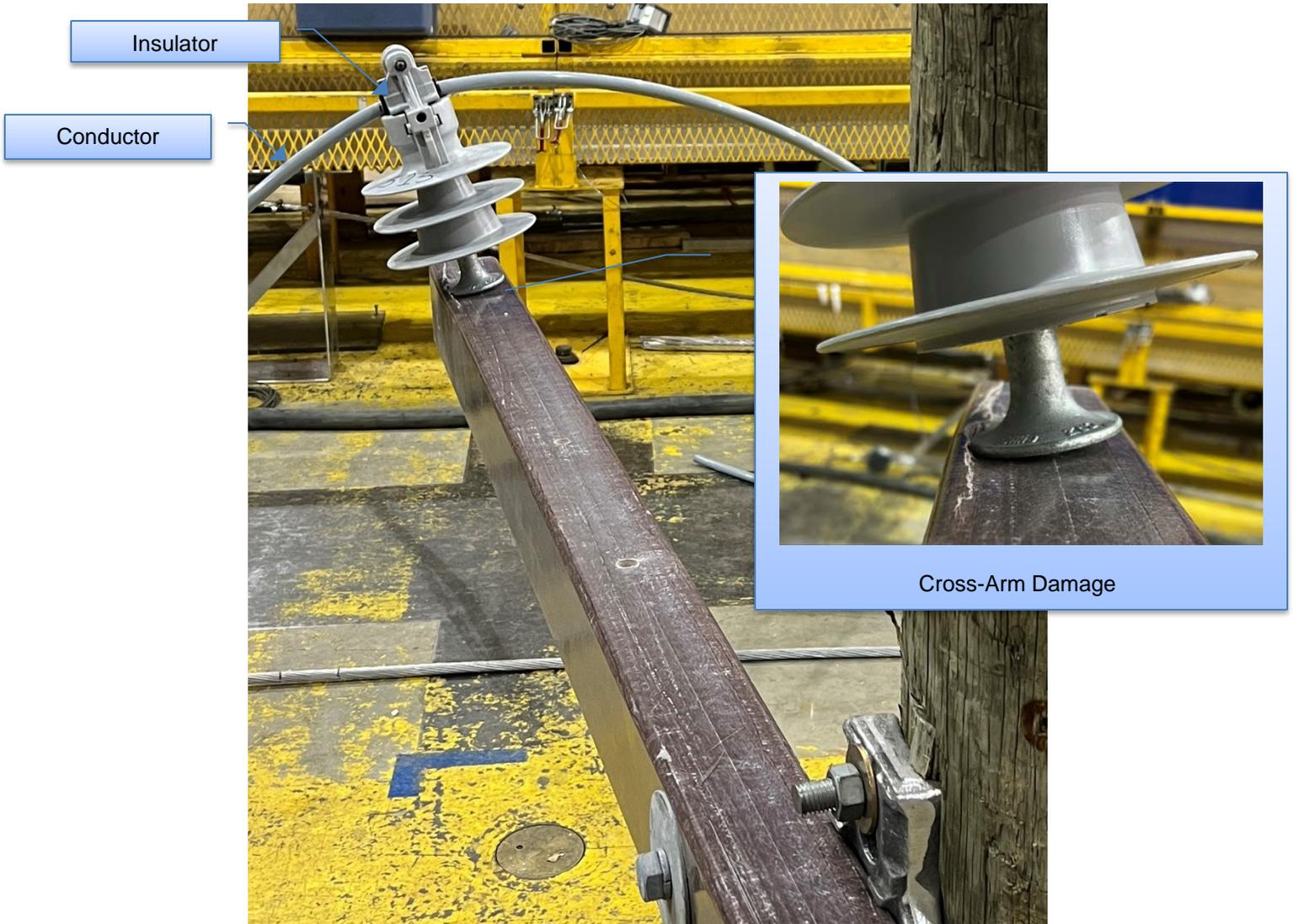
Figure 6-11: Sample 3.1.3 – Insulator and Cross-arm Condition after Test
