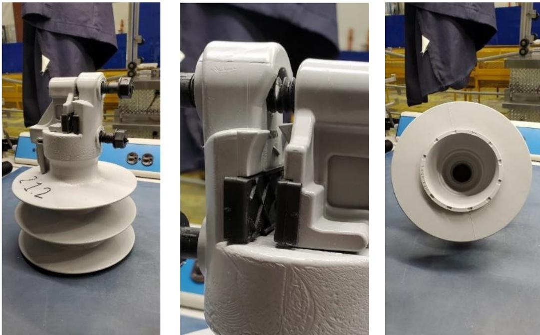
Figure 6-6: [REDACTED] - Typical Insulator Condition after Slip Test (no damage)
