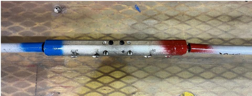
Figure 3-5: [REDACTED] Installed on 15 kV 1/0 AWG, 6/1 ACSR
