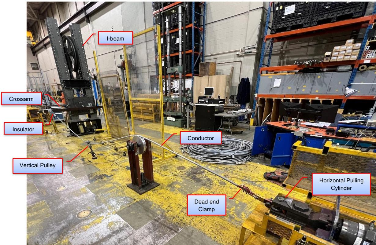
Figure 4-3: Full Mock-up: Picture of the Setup
