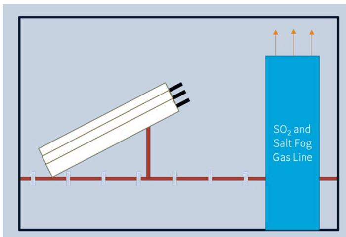
Figure 33. Schematic of salt spray testing apparatus.  $\text{SO}_2$  and 5 wt.% salt fog were introduced through a central tube. Samples were arranged on a plastic platform with grid openings to prevent pooling of runoff. The samples were oriented approximately  $60\text{--}75^\circ$  from vertical.
