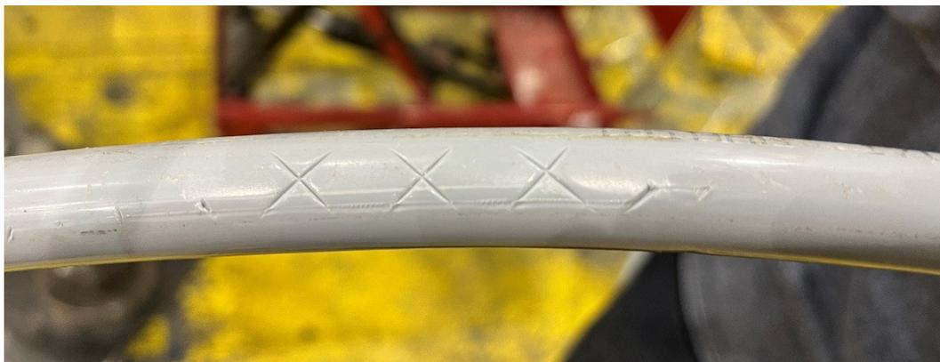
**Figure 6-24: Sample 3.4.3 - 15 kV, 1/0 AWG ACSR Condition after Test**
