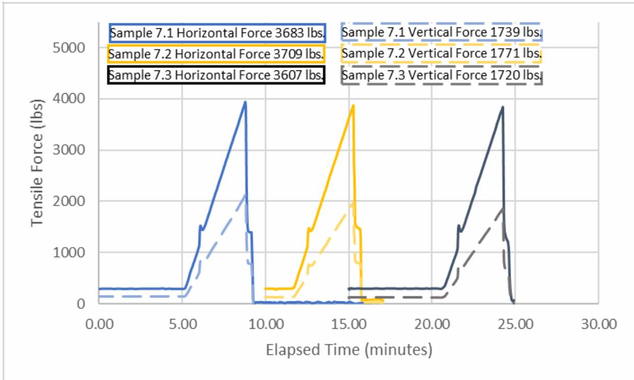
**Figure 6-7: Test Load Profile: 17kV 653.9 KCMIL, 18/3 ACSR Conductor**
