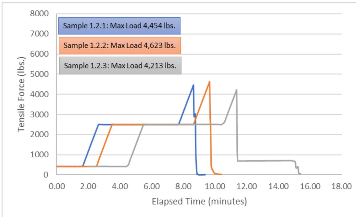
**Figure 6-2: Maximum Load Test – 35 kV, 1/0 AWG ACSR**
