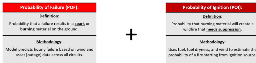
Figure 6-7 Schematic showing the two probability calculations for ignition likelihood and burn probability (fire spread potential)
