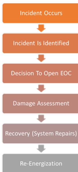
Figure 8-14: Liberty Operational Flow Diagram for Service Restoration
