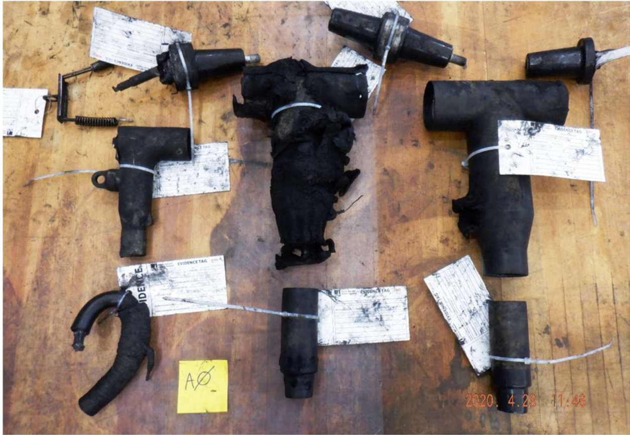
Figure 3: The evidence collected from A phase. The failed tap plug and elbow are shown on the left.
