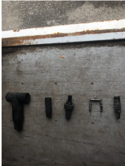
Figure 1-Parts of the damaged connector (collected as evidence)
