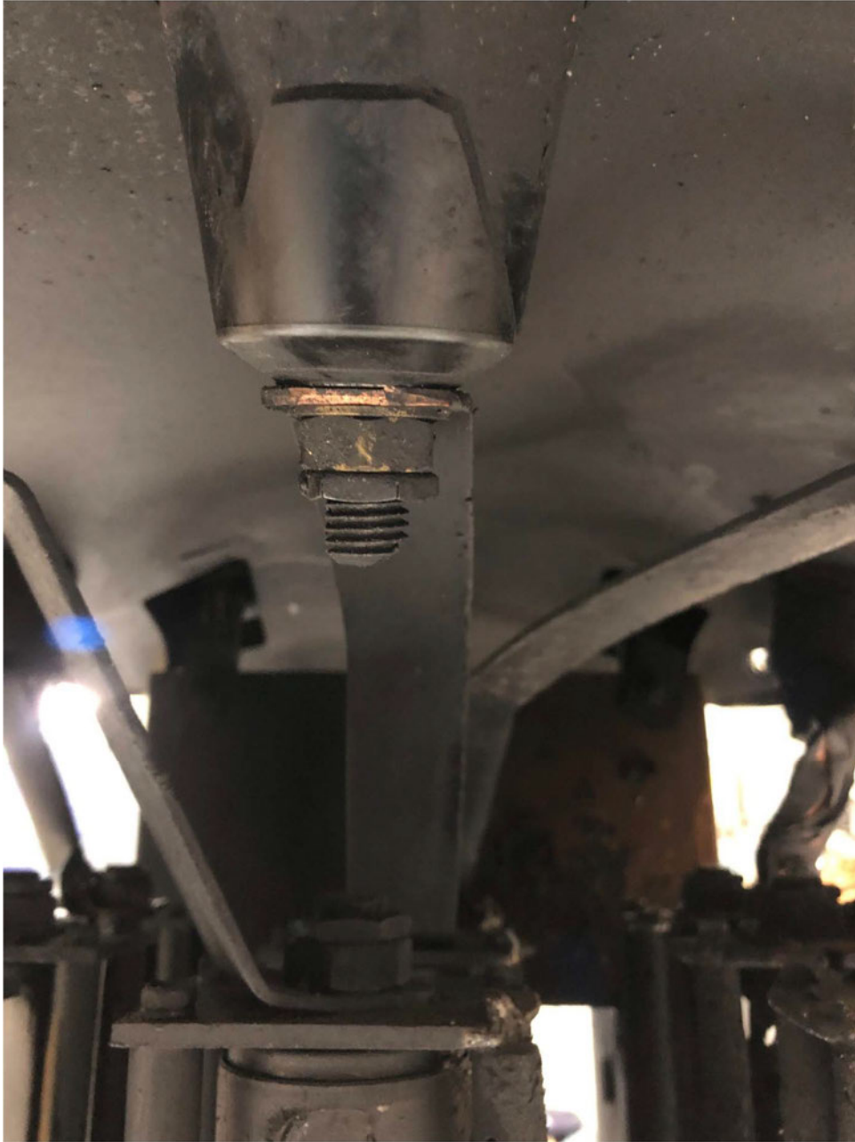
Figure 5: Cracked T2 bushing
