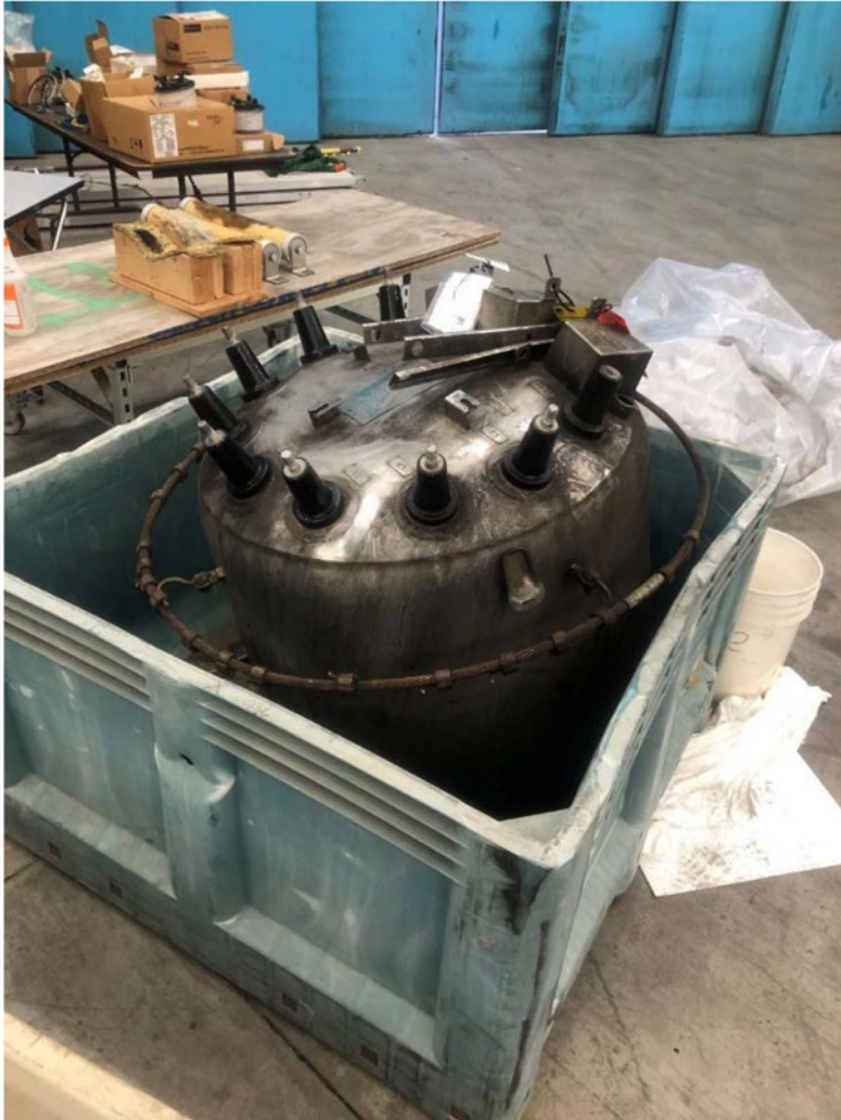
Figure 3: Fire damage evident on tank; burned oil, soot. Switch handles appear to be intact and in the closed position, grounding ring intact and connected to tank.
