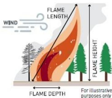
PG&E uses flame length and rate of a fires spread from fire simulations in an operational setting to evaluate the potential need to turn off power. As shown in [Figure PG&E-9.2.1-4](#), flame lengths of 8-11 and >11 poses a serious control problem and therefore, are considered CFB and require a PSPS.
