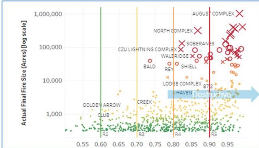
The relationship between the FPI R-score and the historic fire data was examined as well. Destructive fires are denoted by the red X's and plotted with the rate of spread and Flame Length Technosylva simulation results for each wildfire in [Figure PG&E-6.2.2-7](#) below. Thresholds can be drawn for both factors where destructive fires are characterized by a Rate of Spread greater than 12 chains/hour and a Flame Length greater than 5 feet.
