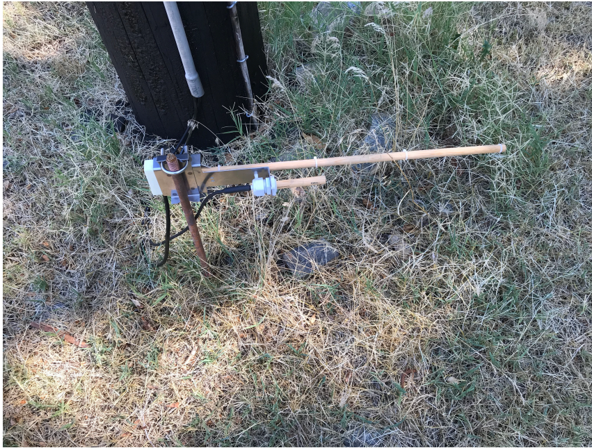
Figure 3—Typical Fuel Monitoring Device
