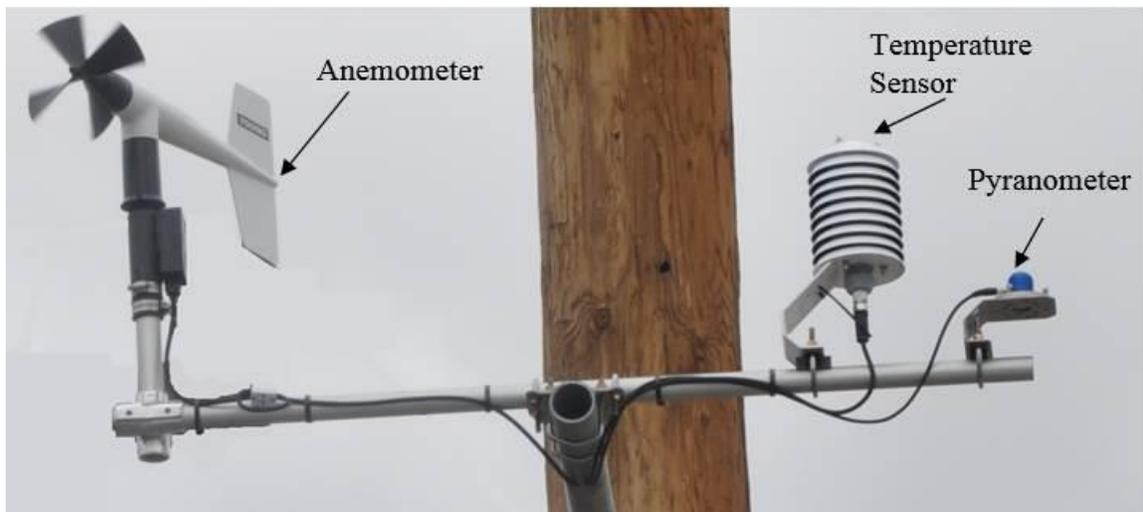
**Additional 2ft crossarm and Rain Gauge not pictured. Pyranometer not applicable to Liberty Utilities Weather Stations. Above picture does not accurately represent final Liberty Utilities weather station crossarm**
