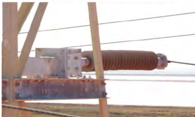
Figure 130 Insulator damage that could result in an A tag (left). The protective sheath has been broken, which would lead to degradation of the core. Damage to insulator sheath, not to the core (right).
