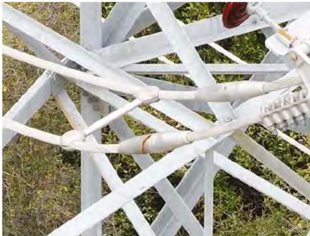
Figure 221 Failed splice (left). Splice is not compressed on one side (right).
