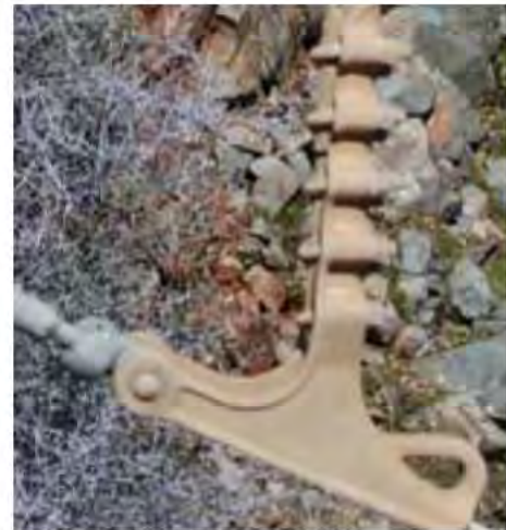
Figure 161 Minor surface rust (left). Hardware surface rust (right): material loss is not significant enough to warrant an E priority notification.
