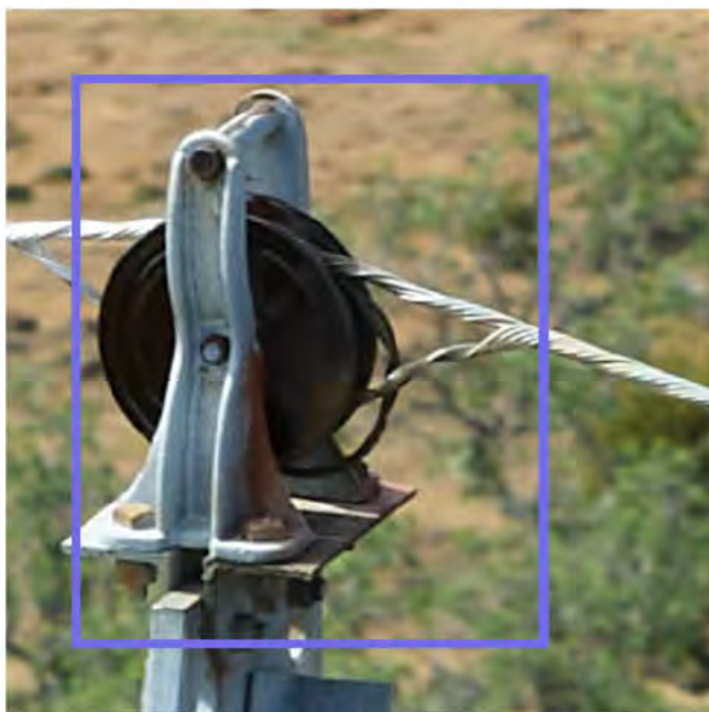
Figure 194 Shield wire block flashed (left) shield insulator flashed (right).
