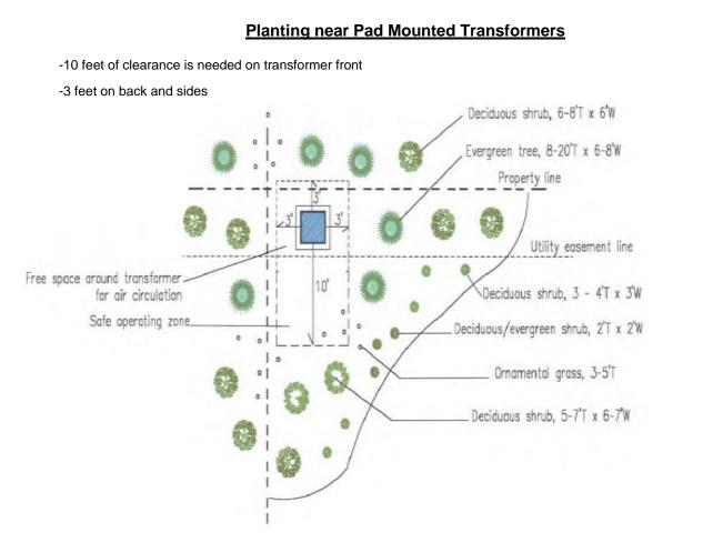
**<u>NOTE</u>**: Pad mounted switches (PME/PMH style etc.) require 10 feet on <u>both</u> front and back to operate. Underground utility high voltage electric boxes/vaults should be located 10 feet from trees to avoid root damage and provide appropriate access.
