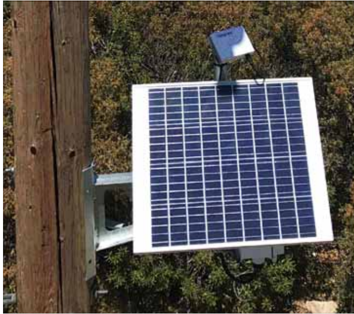
Figure AP 810–6: Typical Installation of Weather Monitoring System (NEMA Enclosure and 65-Watt Solar Panel)
