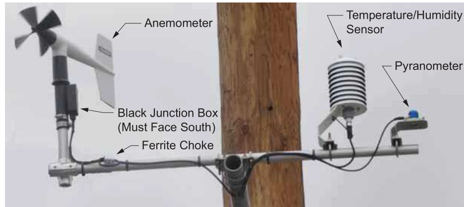
Figure 1125-2: Typical Installation of Weather Monitoring System (Sensors)
