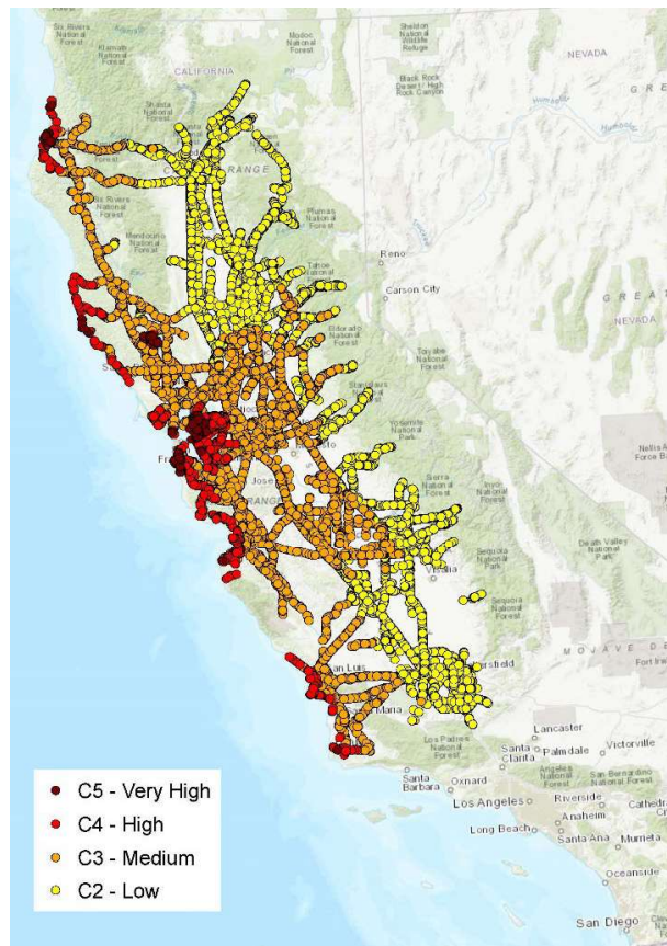
Figure 2.2 Steel Structure Corrosion Categories as determined by the AAC model.
