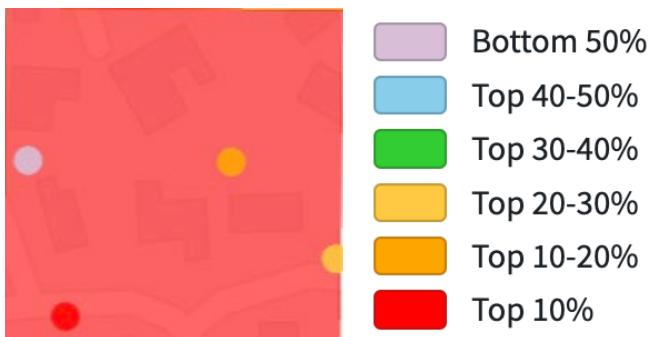
Figure 66. Example pixel for transformer units demonstrating the variability in likelihood of equipment failure within a pixel (from the bottom 50% to the top 10%)
