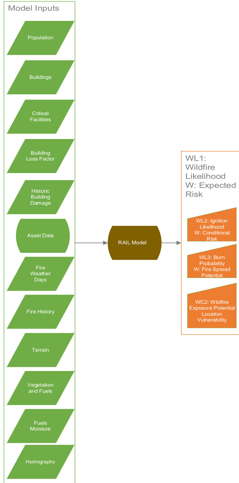
Figure B-1 Risk Associated with Ignition Locations (RAIL) Bowtie Model
