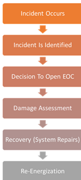
Figure 8-14: Liberty Operational Flow Diagram for Service Restoration
