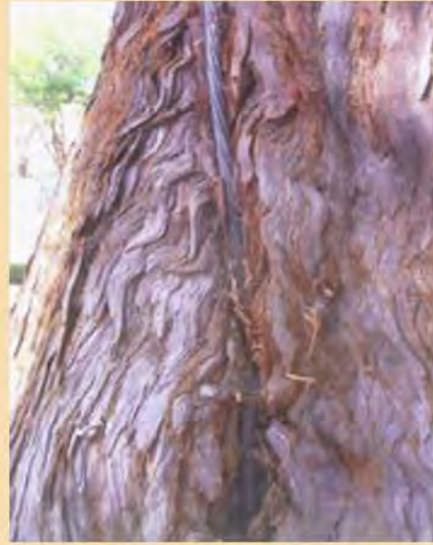
Anchor buried by tree
