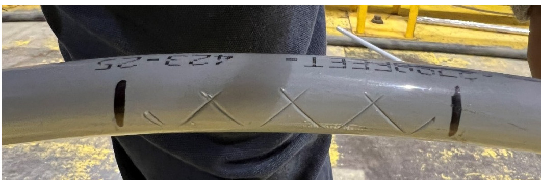
Figure 6-12: Sample 3.1.3 - 17 kV, 1/0 AWG ACSR Condition after Test
