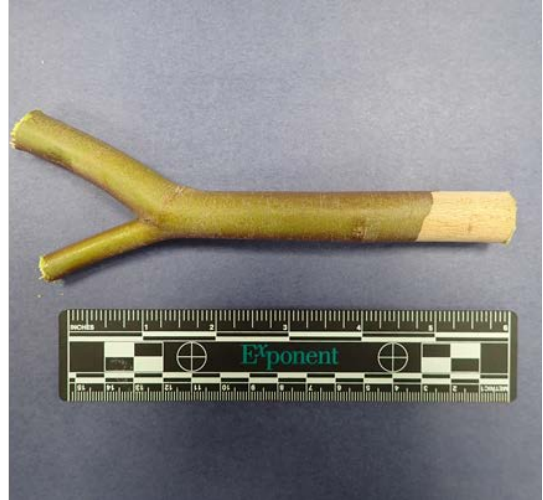
Figure A8. Method for quantifying moisture meter readings and converting to moisture content. The ASTM D4442-20 method of oven-dry mass was used. A fresh branch was cut and weighed, and its moisture content was measured with the moisture meter. The branch was allowed to dry in atmosphere over time. The mass and moisture meter readings were measured over time, until the mass of the branch was constant, indicating that the oven-dry mass was reached. Moisture meter readings above 5 (MC \approx 60%) were considered to be valid for phase-to-phase contact tests.
