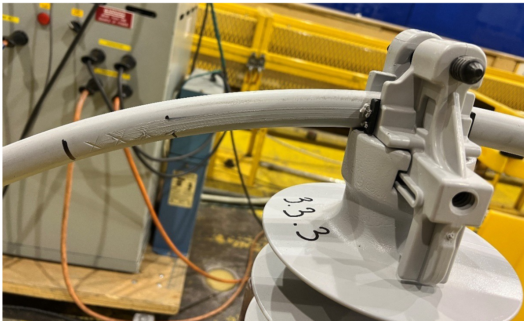
Figure 6-20: Sample 3.3.3 - 22 kV, 397.5 kcmil AAC Condition after Test
