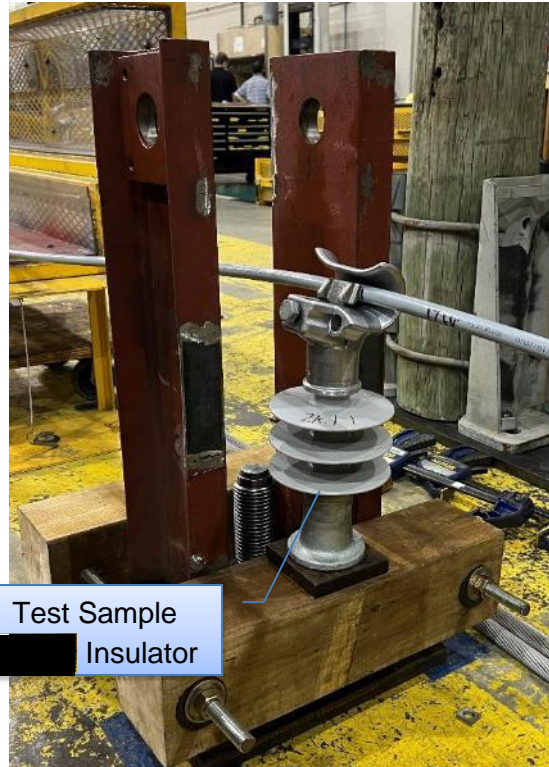
Figure 4-2: Clamp Slip Test Setup
