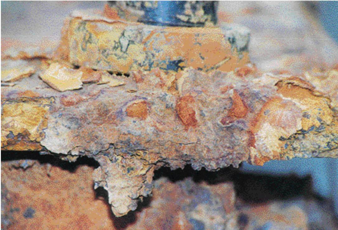
**Figure 5-6: Heavy Corrosion — Example 3 of 3**
