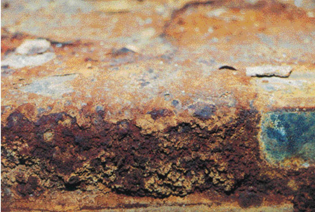
Figure 5–9: Moderate Corrosion — Example 3 of 3
