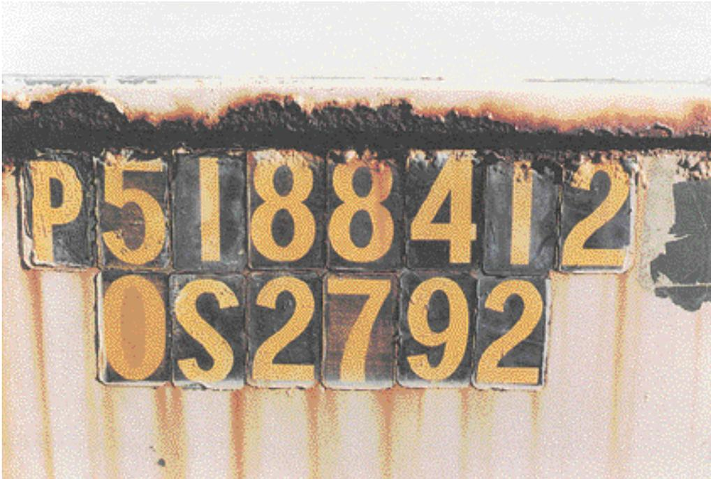
Figure 6–15: Loss of Metal
