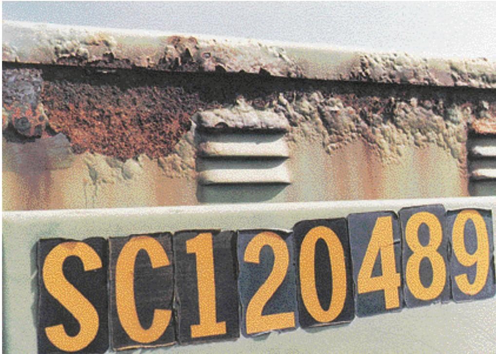
**Figure 6–7: Distinct Corrosion of Component Structural Support Members**
