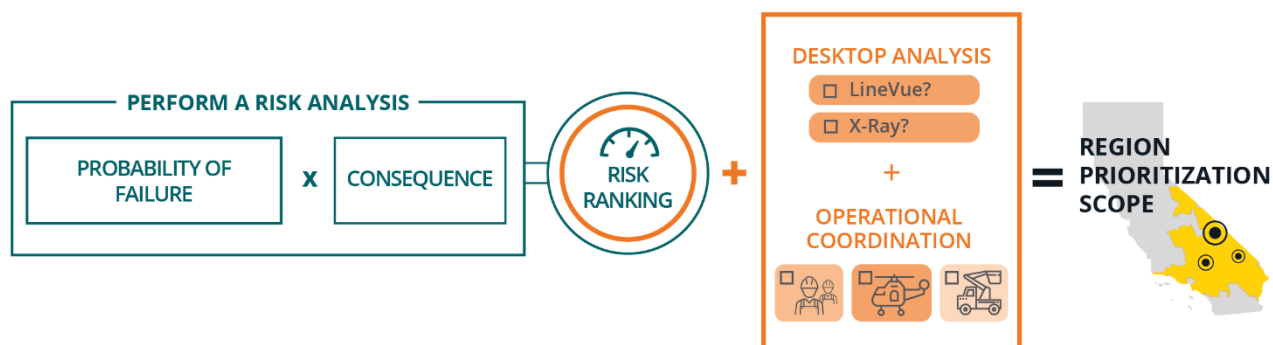
Figure SCE 8-34 - Transmission Conductor and Splice Prioritization
