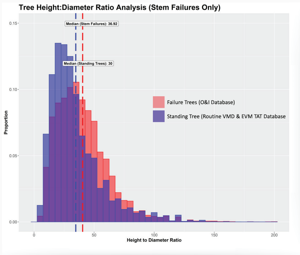
— FIGURE F2. Height to diameter ratio distribution comparison of stem failure trees against all standing trees.
