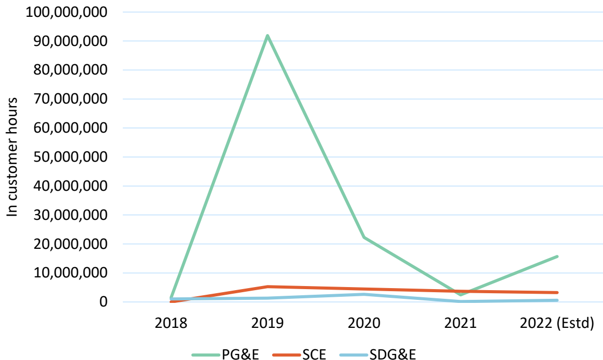
Figure 4.7-4: Recent Use of PSPS: Duration of PSPS Events (Total) – Large IOUs (2018-2021 Actual, 2022 Estimated) 212
