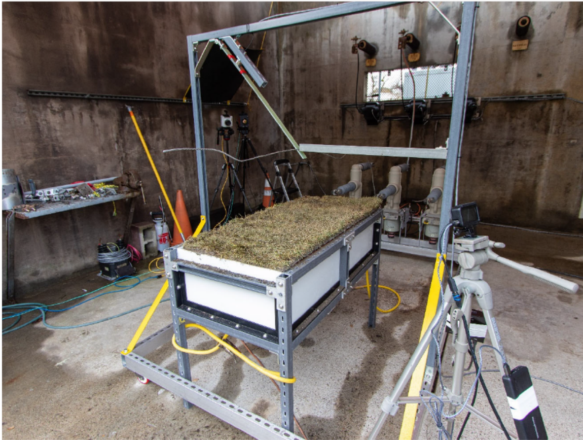
Figure 2: Line-to-ground test apparatus
