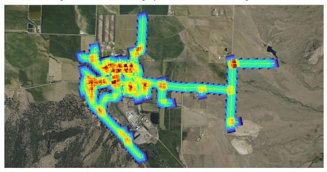
Figure 4.5-1: Conductor Length per Unit Area After Smoothing
