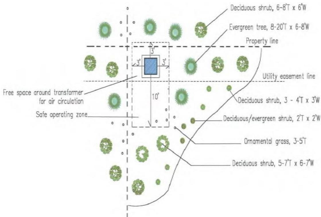
**NOTE:** Pad mounted switches (PME/PMH style etc.) require 10 feet on both front and back to operate. Underground utility high voltage electric boxes/vaults should be located 10 feet from trees to avoid root damage and provide appropriate access.
