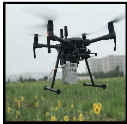
PHOTO 4 LiAIR V70 LIDAR MAPPING SYSTEM
