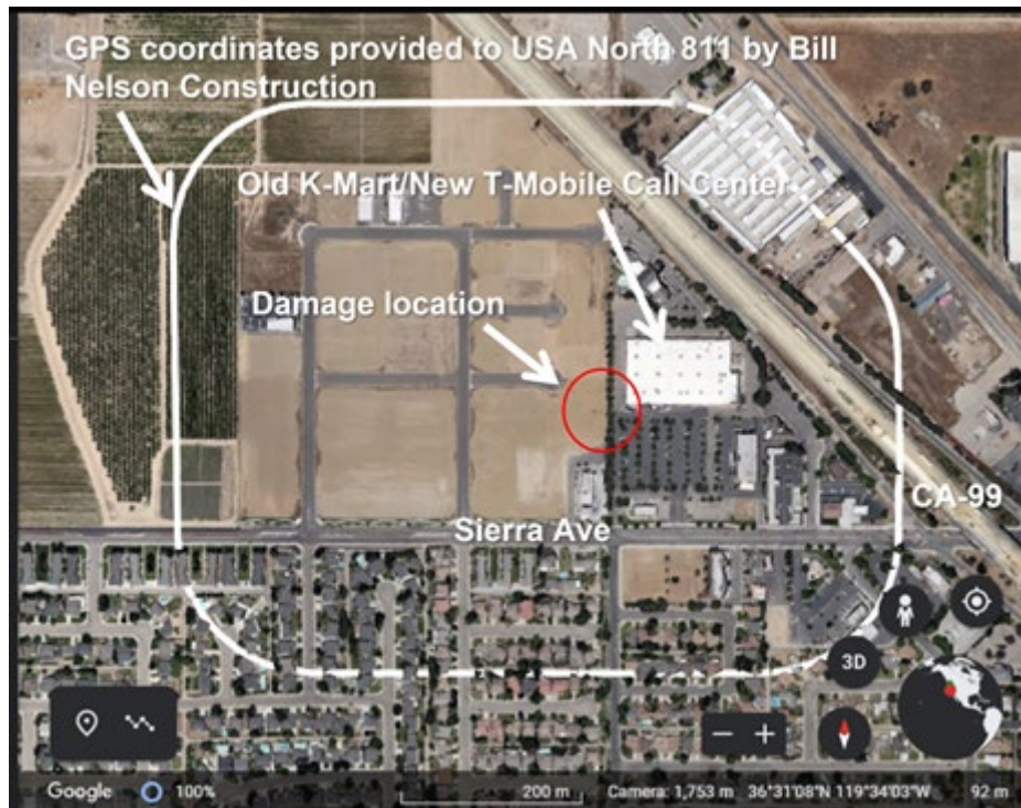
Figure 1. Google Earth map image of excavation polygon submitted by Bill Nelson Construction (Ticket # X114000542-00X) and approximate damage location, Kingsburg, CA. Excavation polygon includes 200-foot buffer added by USA North 811.
