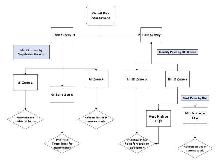
Figure 7.1-1: Flow Chart for Circuit Risk Determination and Prioritizing WMP Work
