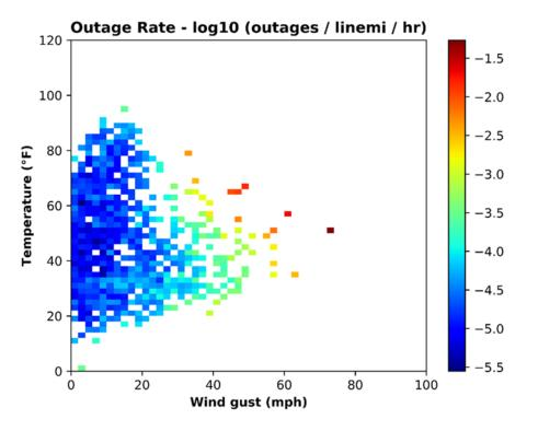
Figure 4.4- 4: Outage Rate in Wind and Temperature Bins
