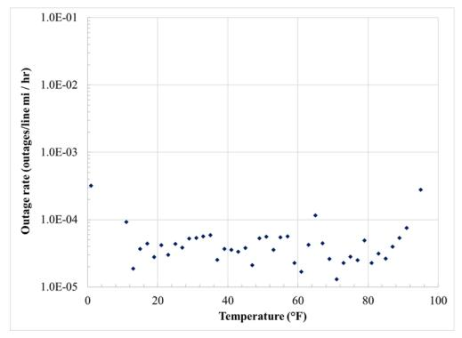
Figure 4.4- 5: Outage Rate as a Function of Temperature Independent of Wind Gust
