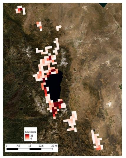
Figure 4.4- 2: Overhead line miles density on RTMA grid
