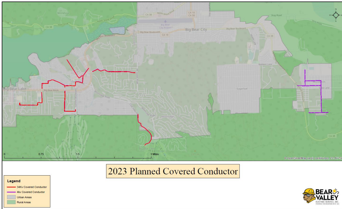
Figure 7.3-5: 2023 Planned Covered Conductor Installation Location
