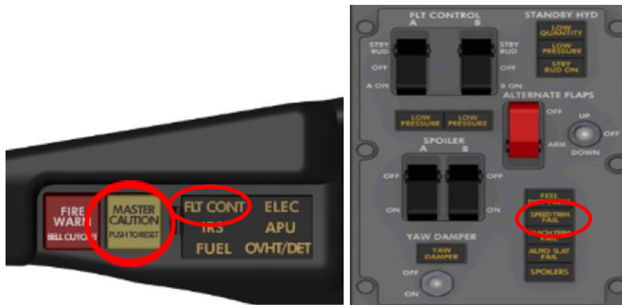
FIGURE 2 SPEED TRIM FAIL ANNUNCIATION
