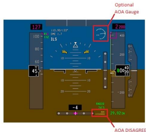
FIGURE 4 737 MAX MDS PFD WITH AOA DISAGREE AND AOA GAUGE
