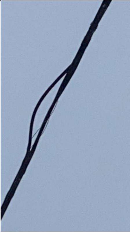
Item9CD4Img1: Broken support strand
